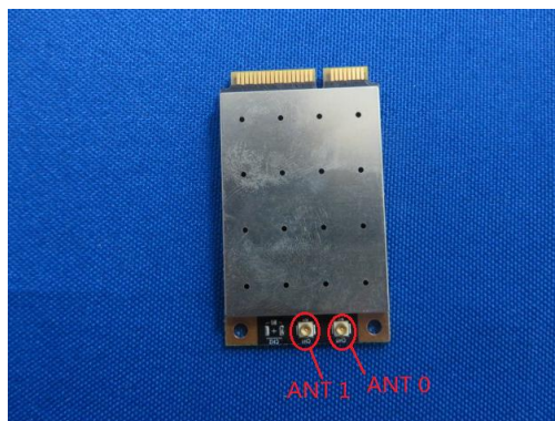
Antenna RF Port Plot
