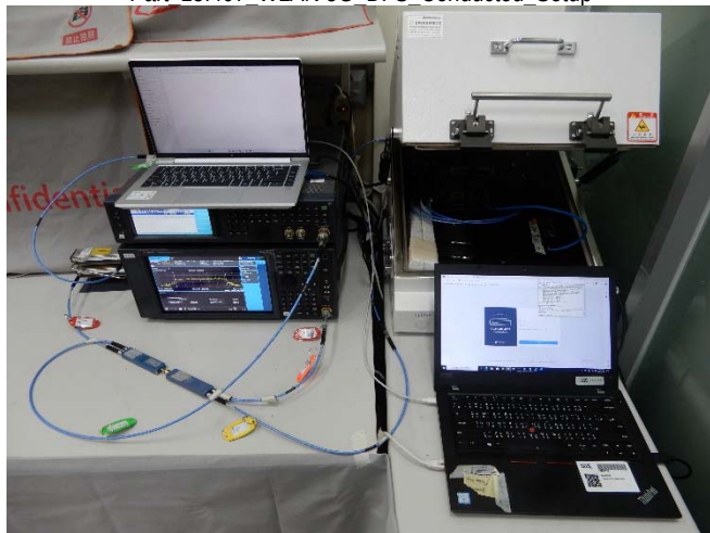
Part 15.407 WLAN 5G DFS Conducted Setup
