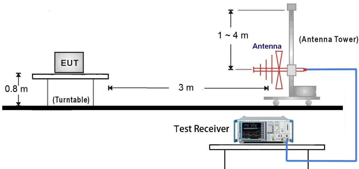
1GHz ~18GHz Test Setup:
