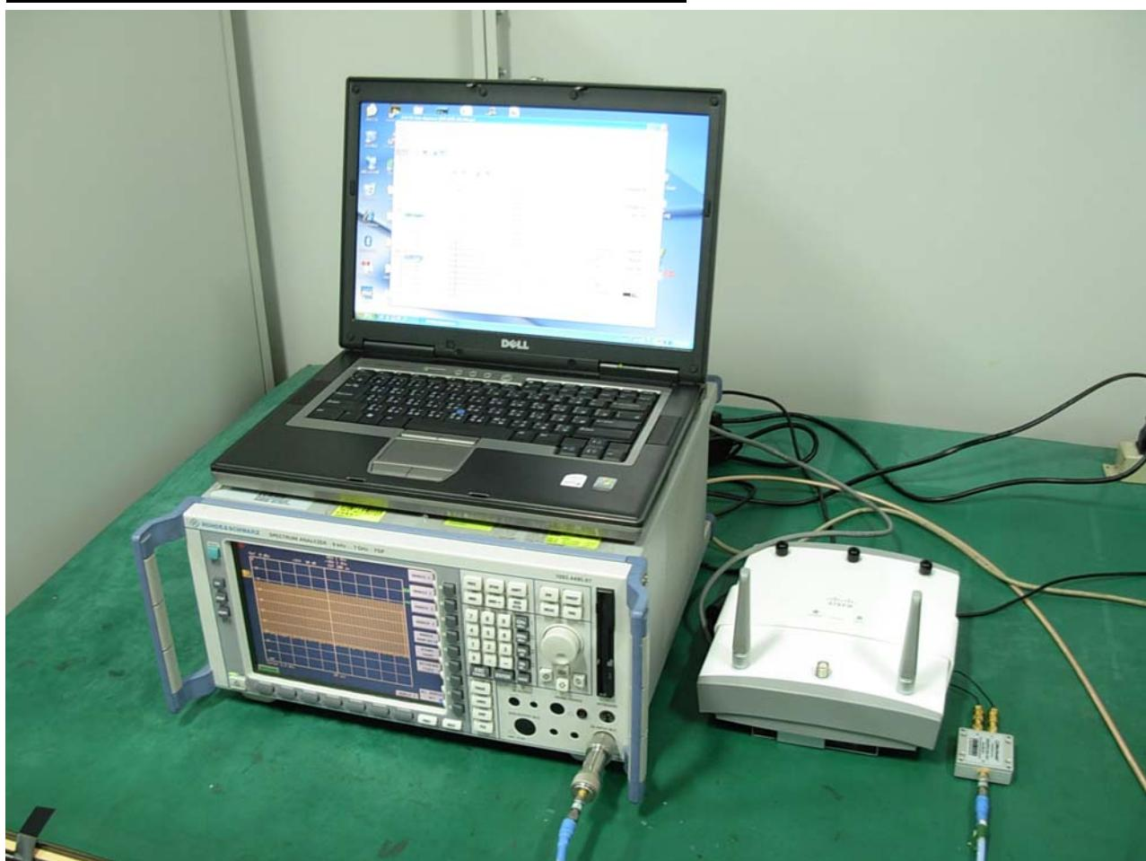
**DFS Set-up Photo: Client and Radar Generator**
