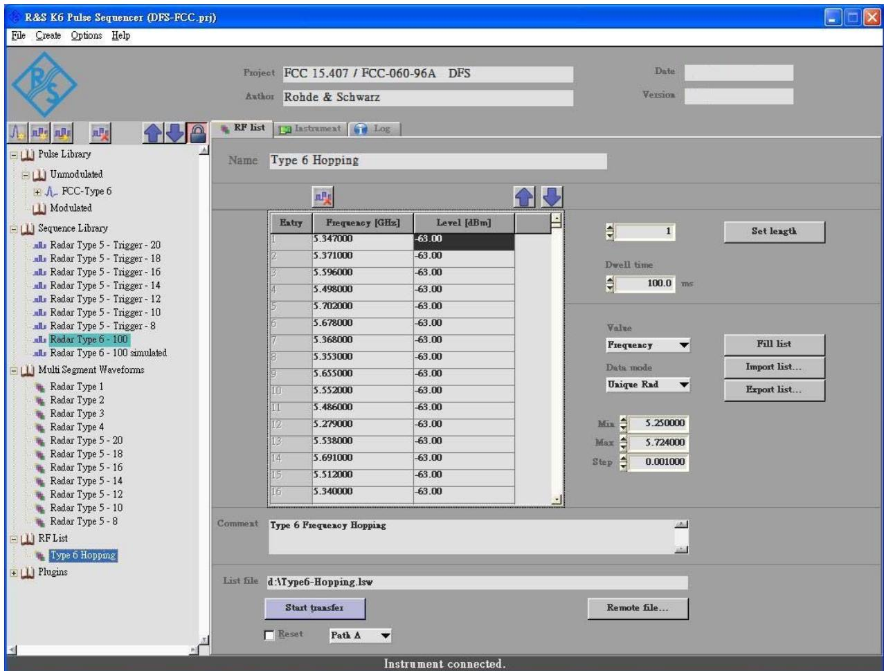
Used R&S Pulse K6 Sequencer Software to select the waveform parameters from the bounds of the signal type, system were random selection using uniform distribution.
