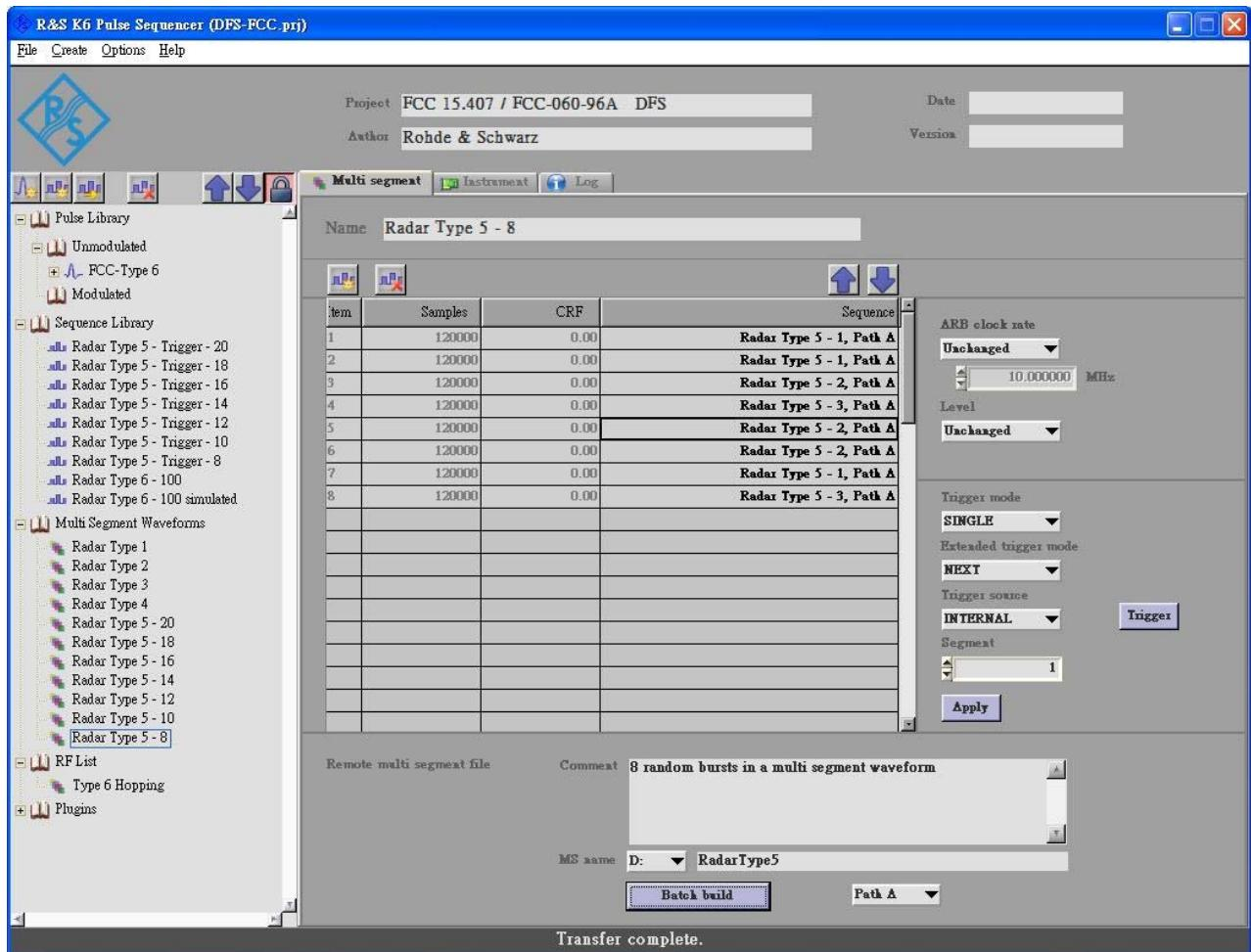
Used R&S K6 Pulse Sequencer Software to select the waveform parameters from the bounds of the signal type, system were random selection using uniform distribution.
