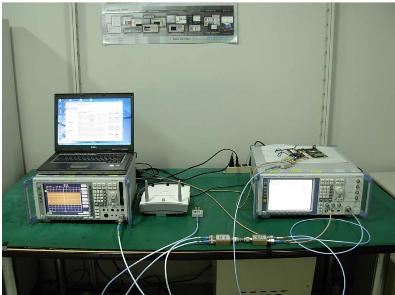
**DFS Set-up Photo: Master and Spectrum Analyzer**
