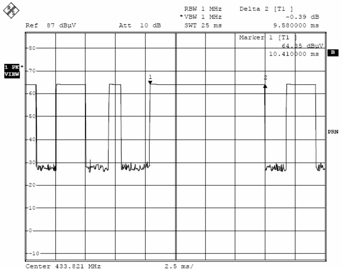
The graph shows the duration of long 'on' signal. From marker 1 to marker 2, duration is 9.58ms.
