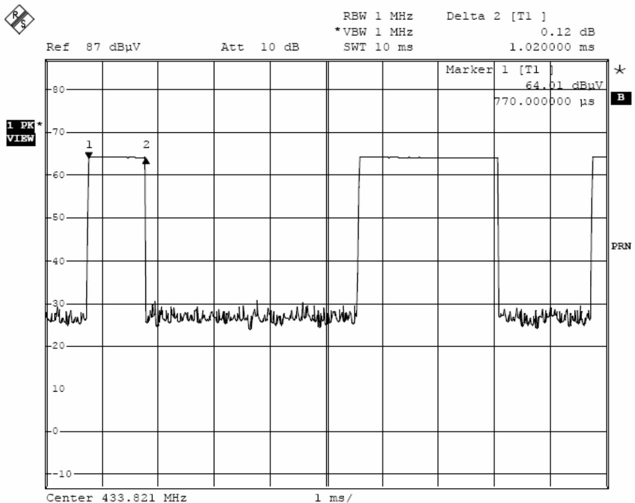
The graph shows the duration of short 'on' signal. From marker 1 to marker 2, duration is 1.02ms.
