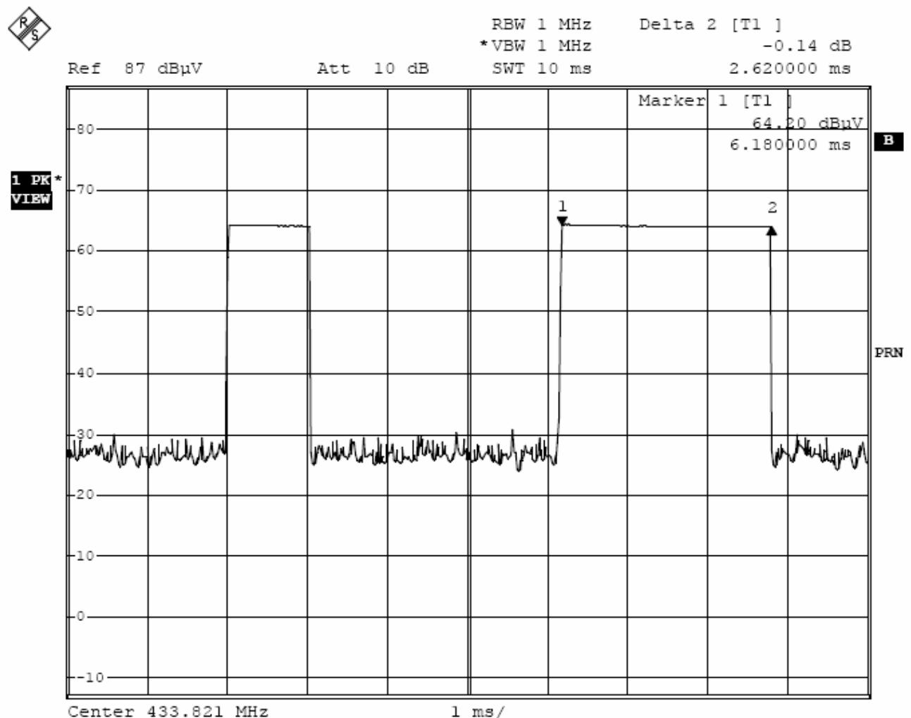
The graph shows the duration of middle 'on' signal. From marker 1 to marker 2, duration is 2.62ms.
