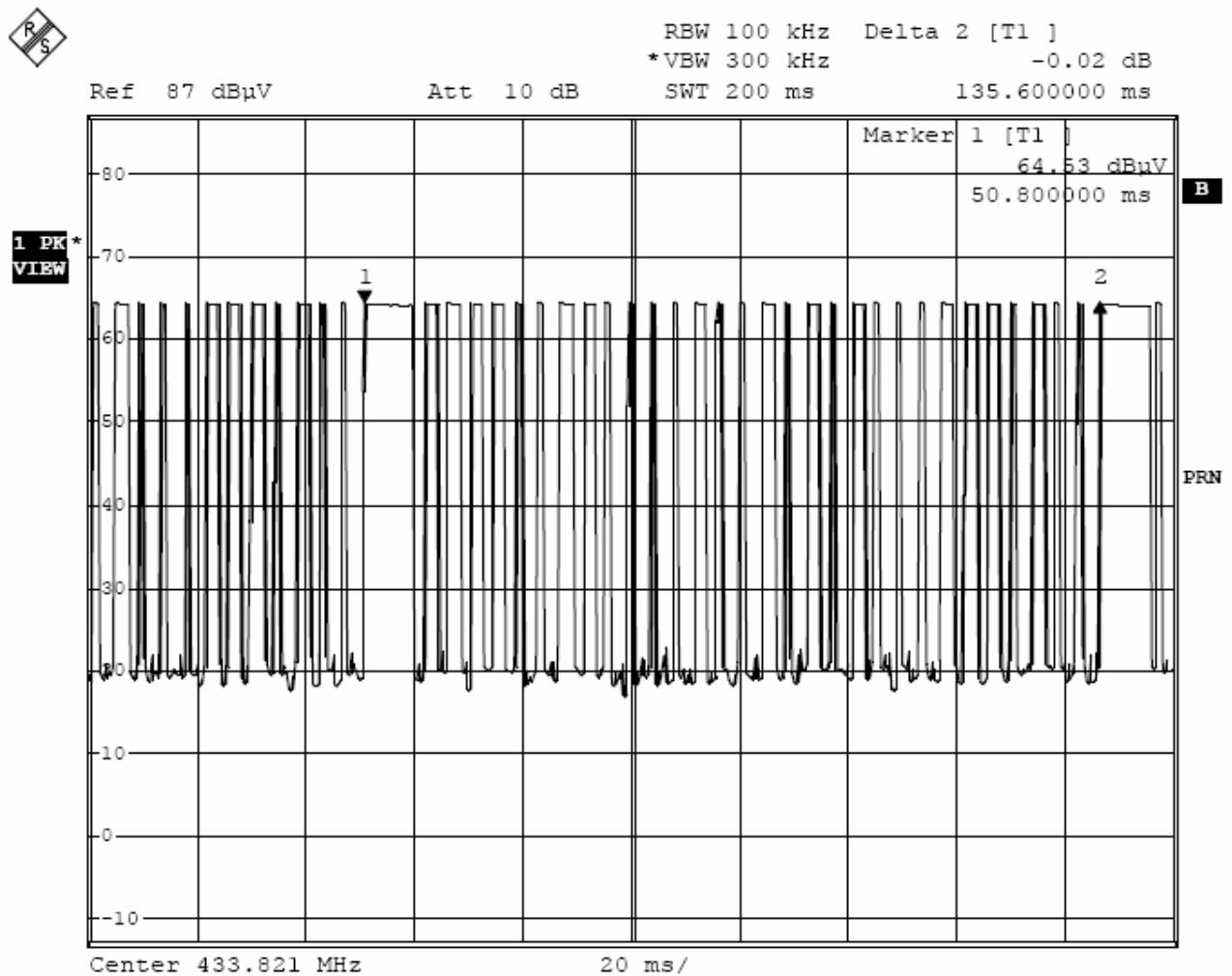
The graph shows the pattern of coding during the signal transmission. The time interval of one coding period starts from marker 1 to marker 2, Hence the total time of one period is 135.6ms. It sums of 1 long 'on' signals and 14 middle 'on' signals and 16 short 'on' signals.
