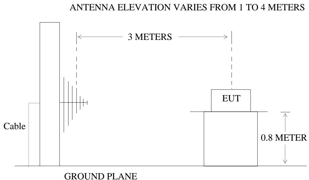
(EUT: Wireless Analog Outdoor Temperature / Humidity Transmitter)
