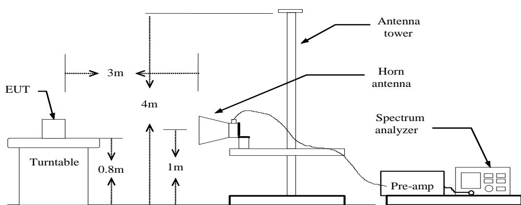
Above 10 GHz shall be extrapolated to the specified distance using an extrapolation factor of 20 dB/decade from 3m to 1.5m.
