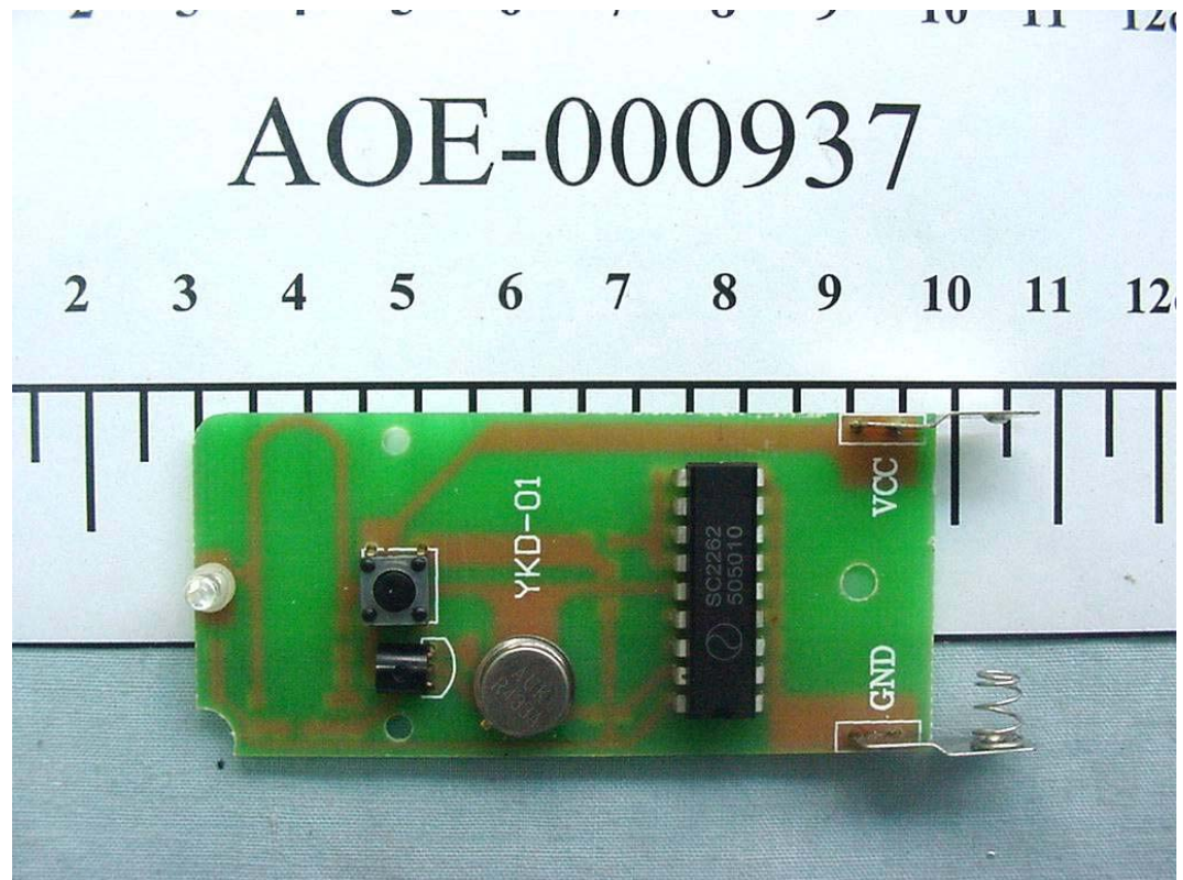
FIGURE 3 RF TIMER CONTROLLER (M/N: 5244341H) MAIN BOARD (COMPONENT SIDE)
