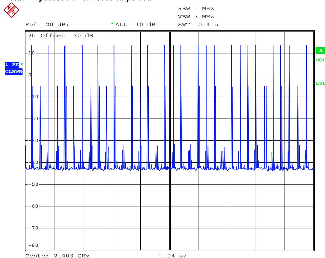
**Test Mode: Channel Low****A single pulse is 0.8ms**
