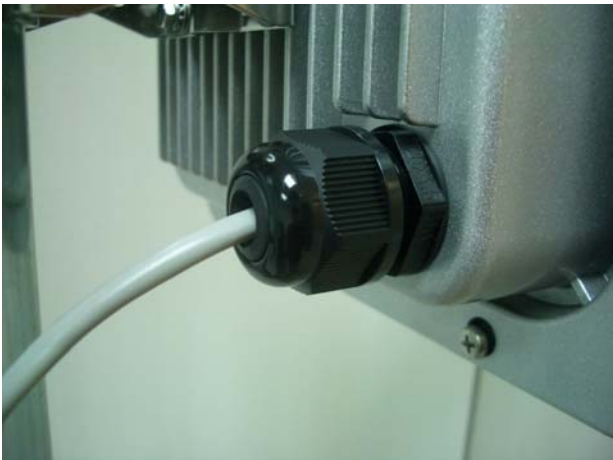
Step 2: Ethernet cable to connect POE Splitter set
