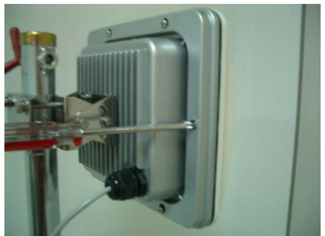
Step 5: To screw the housing
