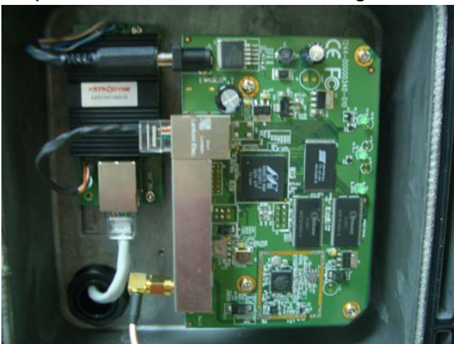
Step 4: Antenna to connect AP/Bridge
