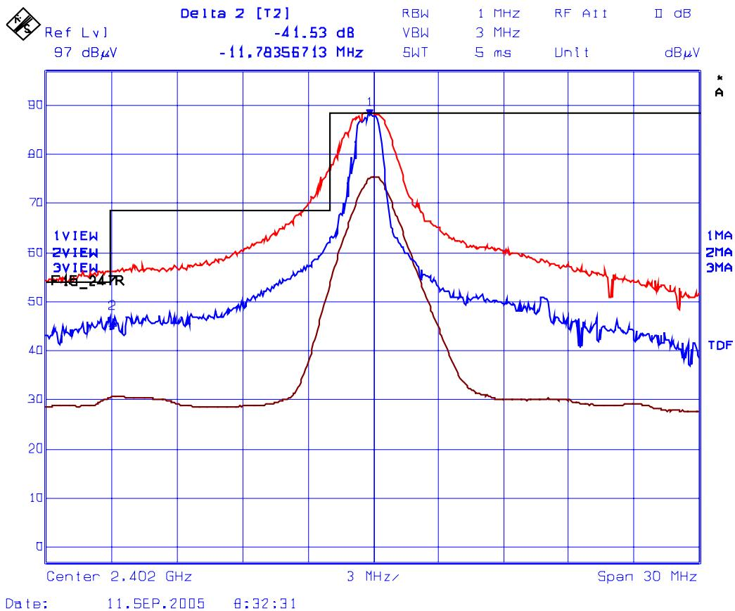
Plot 17: Band-Edge RF Radiated Emissions, Horizontal Polarization
