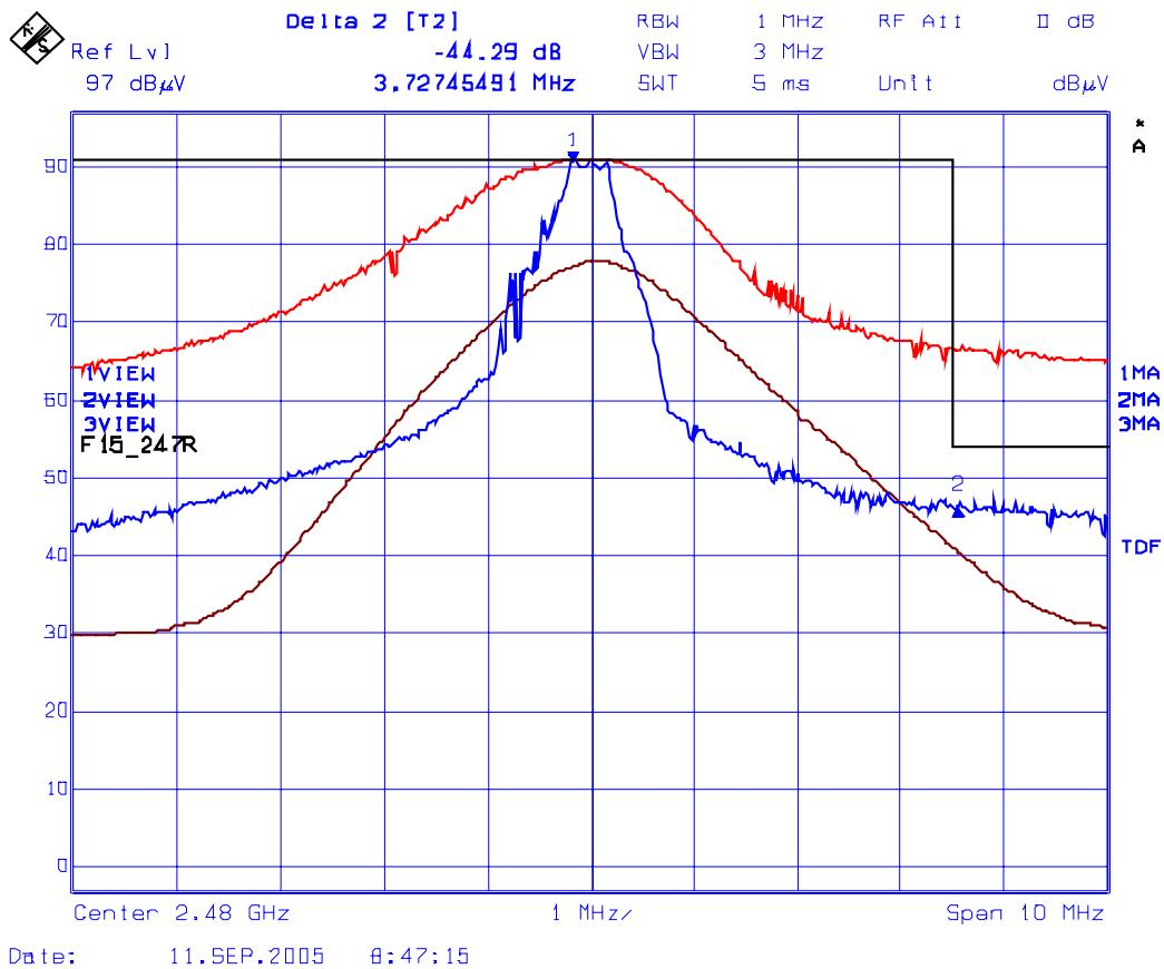
Plot 19: Band-Edge RF Radiated Emissions, Horizontal Polarization
