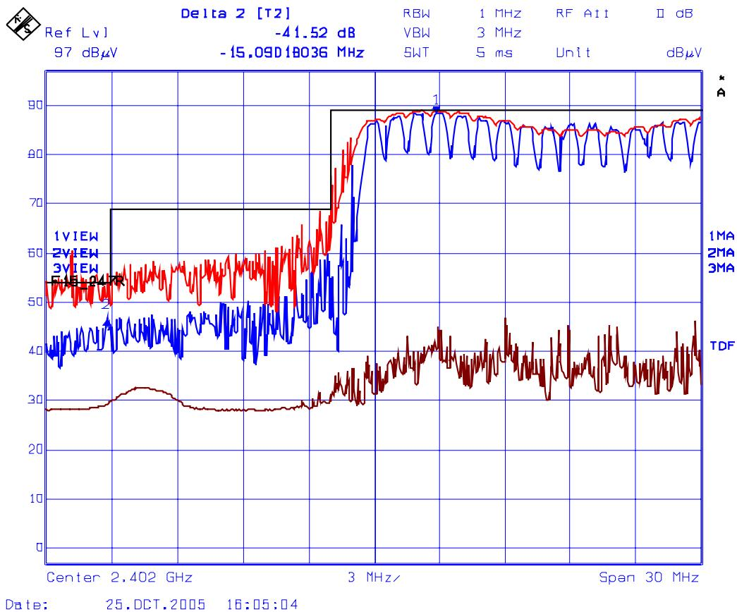
Plot 21: Band-Edge RF Radiated Emissions, Horizontal Polarization
