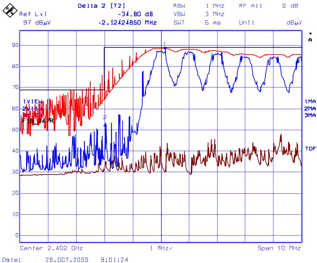
Plot 20: Band-Edge RF Radiated Emissions, Vertical Polarization
