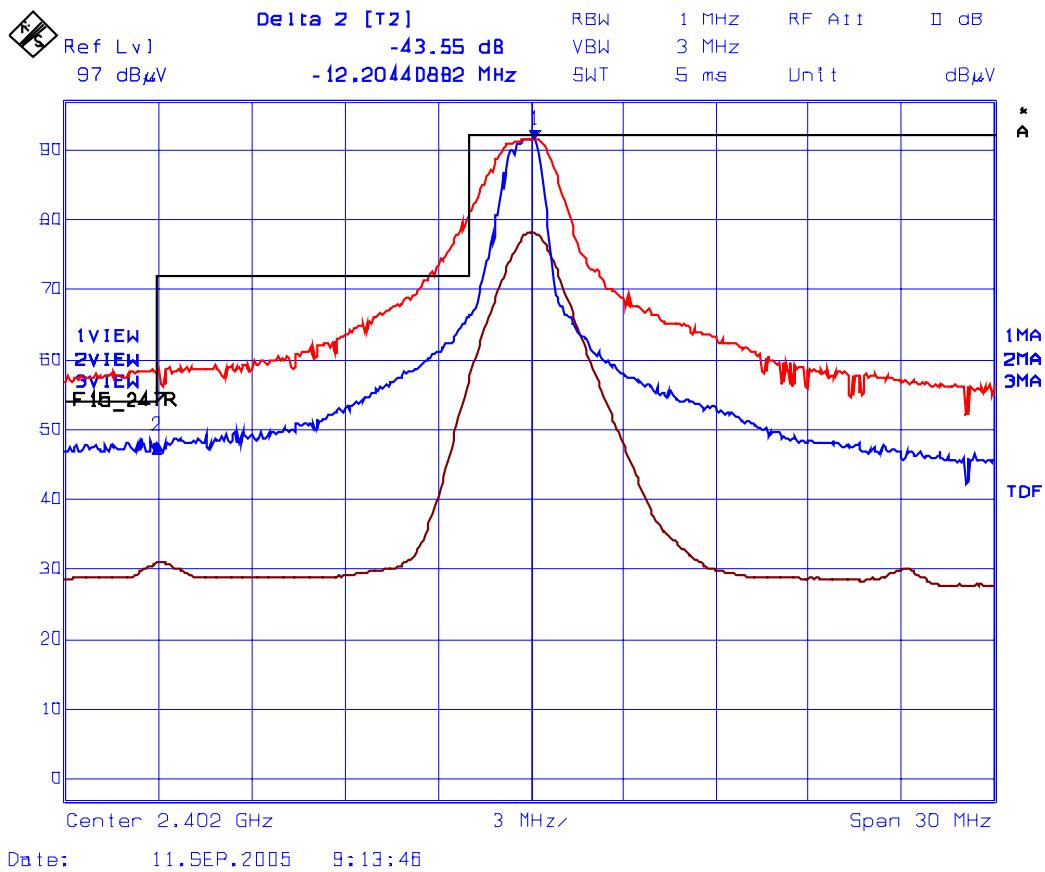
Plot 16: Band-Edge RF Radiated Emissions, Vertical Polarization
