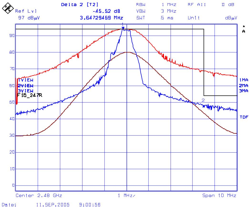
Plot 18: Band-Edge RF Radiated Emissions, Vertical Polarization
