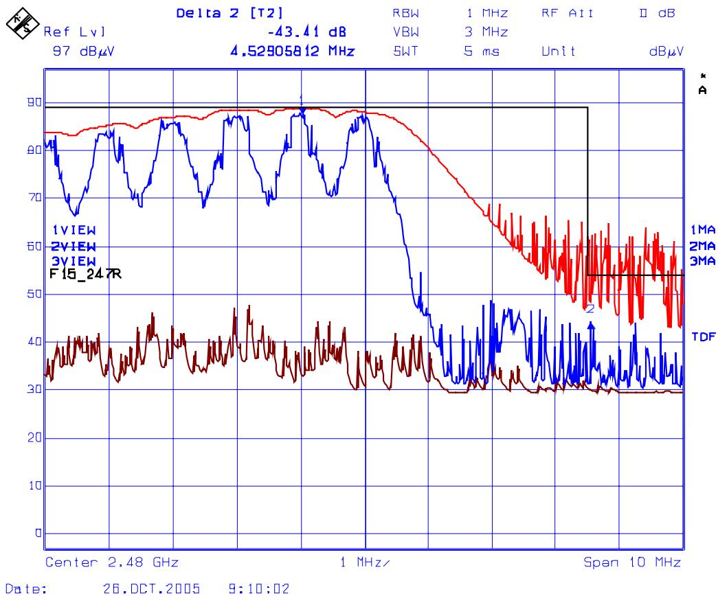
Plot 22: Band-Edge RF Radiated Emissions, Vertical Polarization
