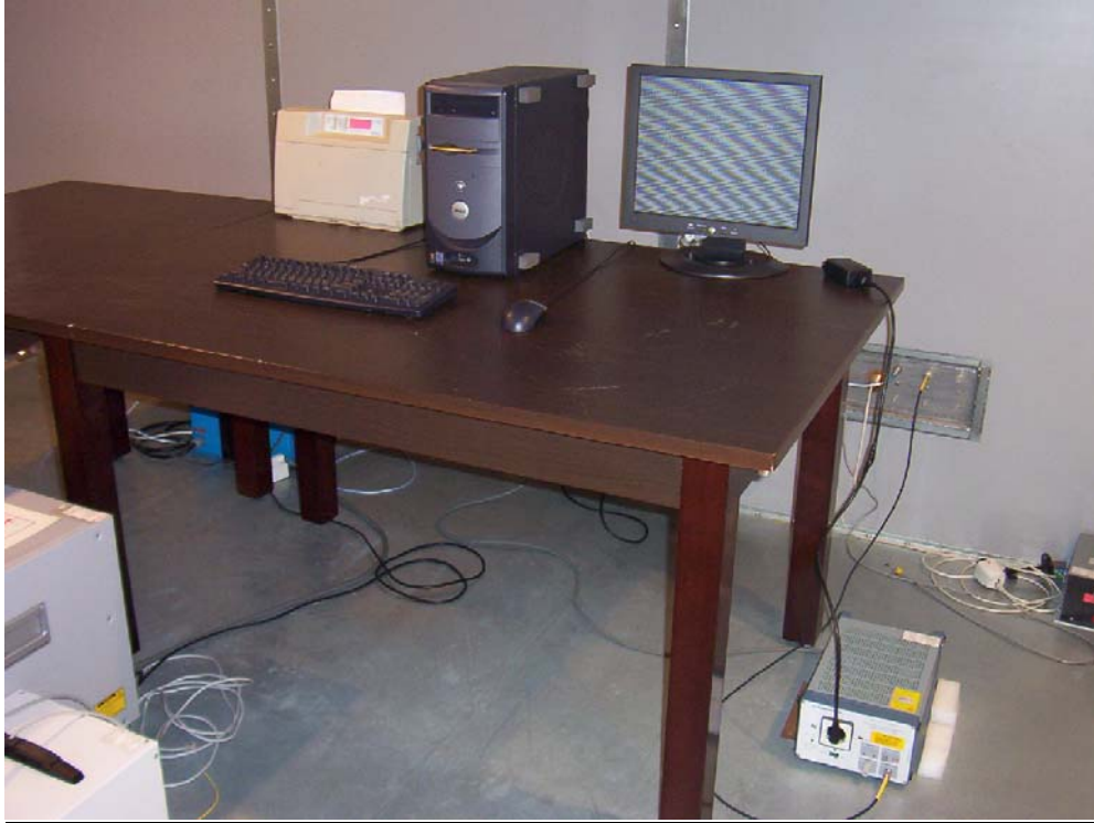
Conducted emission test (Rear)
