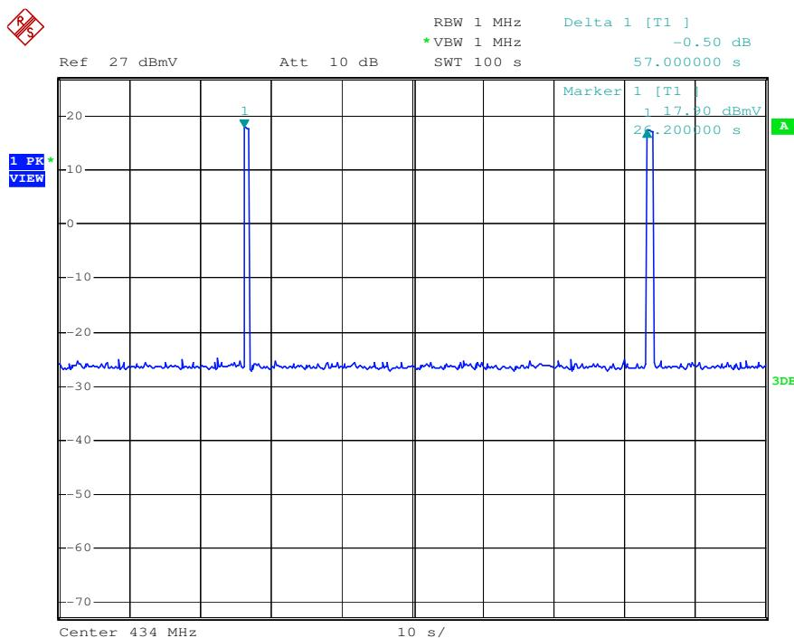
**The results: The unit does meet the FCC Part 15C Section 15.231 requirements.**
