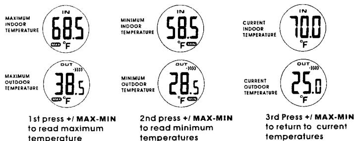
When **MAXIMUM** or **MINIMUM** indoor and outdoor temperatures are displayed, press **CLEAR** to reset both. The readout will appear as "----" and will start to record again.
