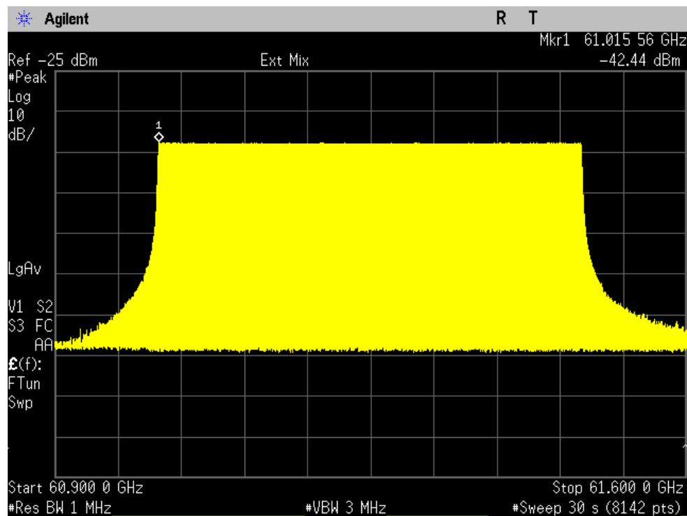
**61 - 61.5 GHz\_ Avg det\_Ant+Amp+Presel\_1 MHz RBW\_30 sec sweep**
