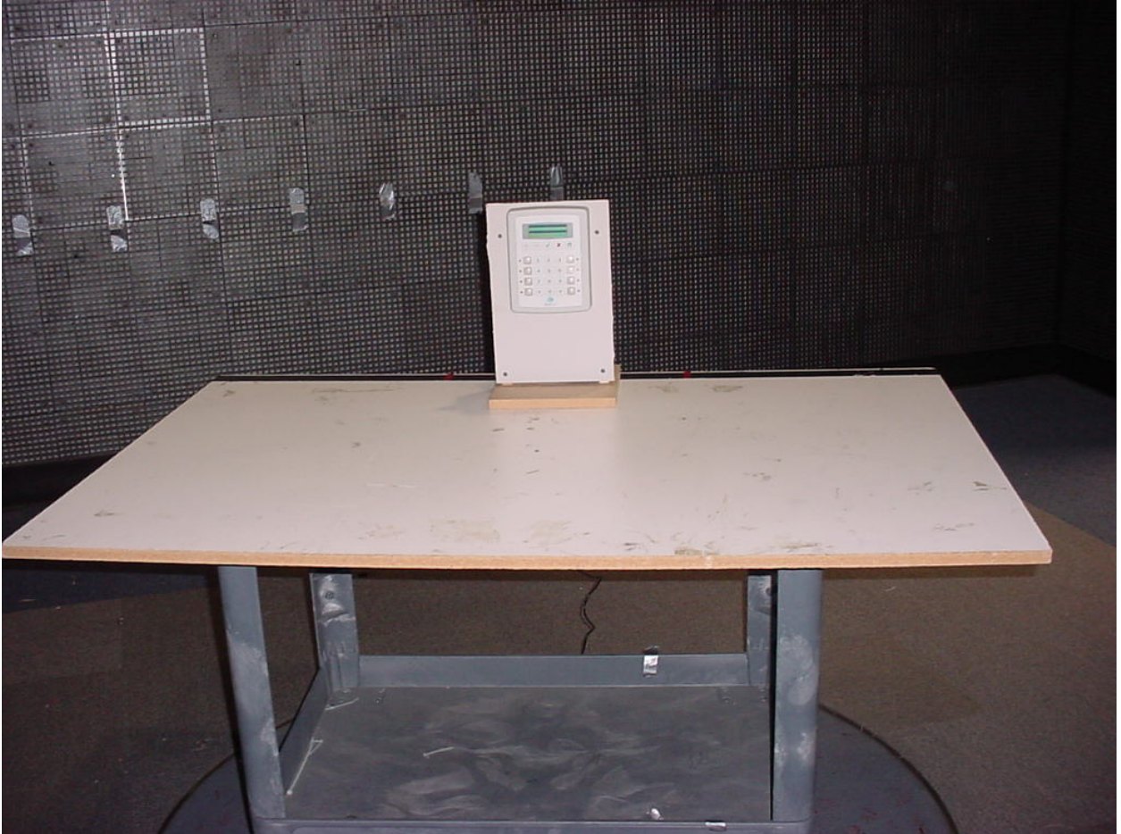
Figure 3: Test Setup – Radiated Emissions
