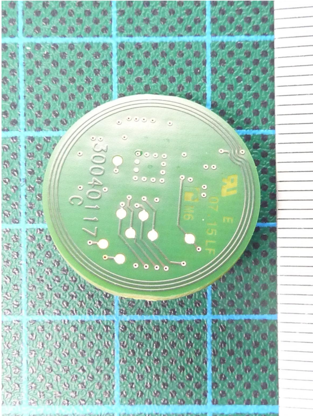
161791pcbG2.jpg: EUT (Excellence Titrator T9), PCB 7, 13.56 MHz RFID reader, bottom view
