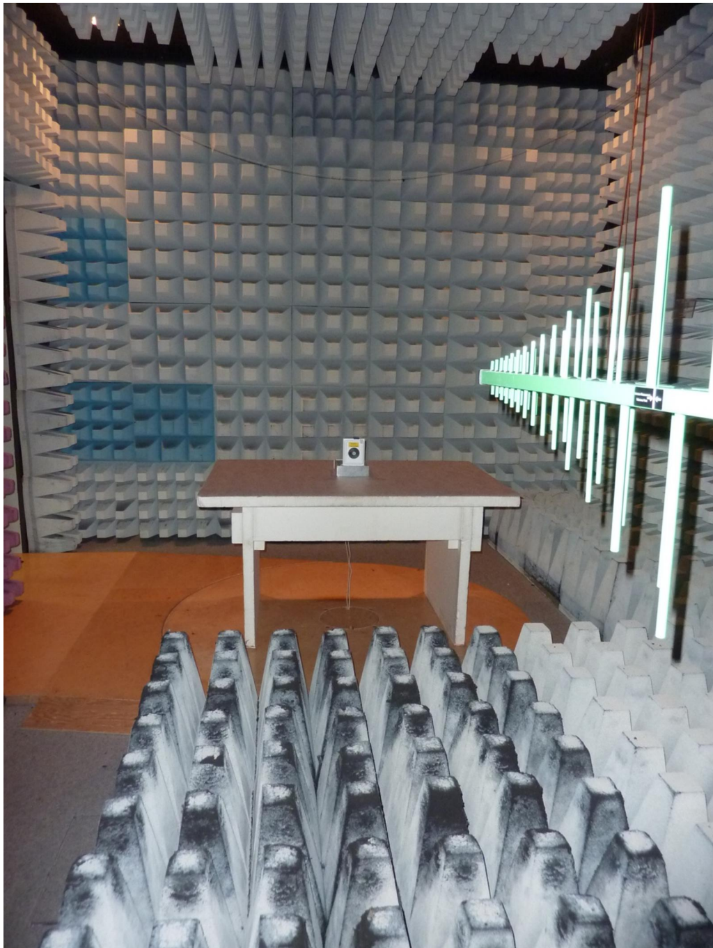
172416_9.jpg: SmartScan, test set-up fully anechoic chamber
