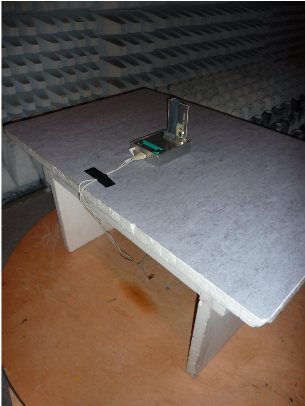
172416_6.jpg: SmartScan, test set-up fully anechoic chamber
