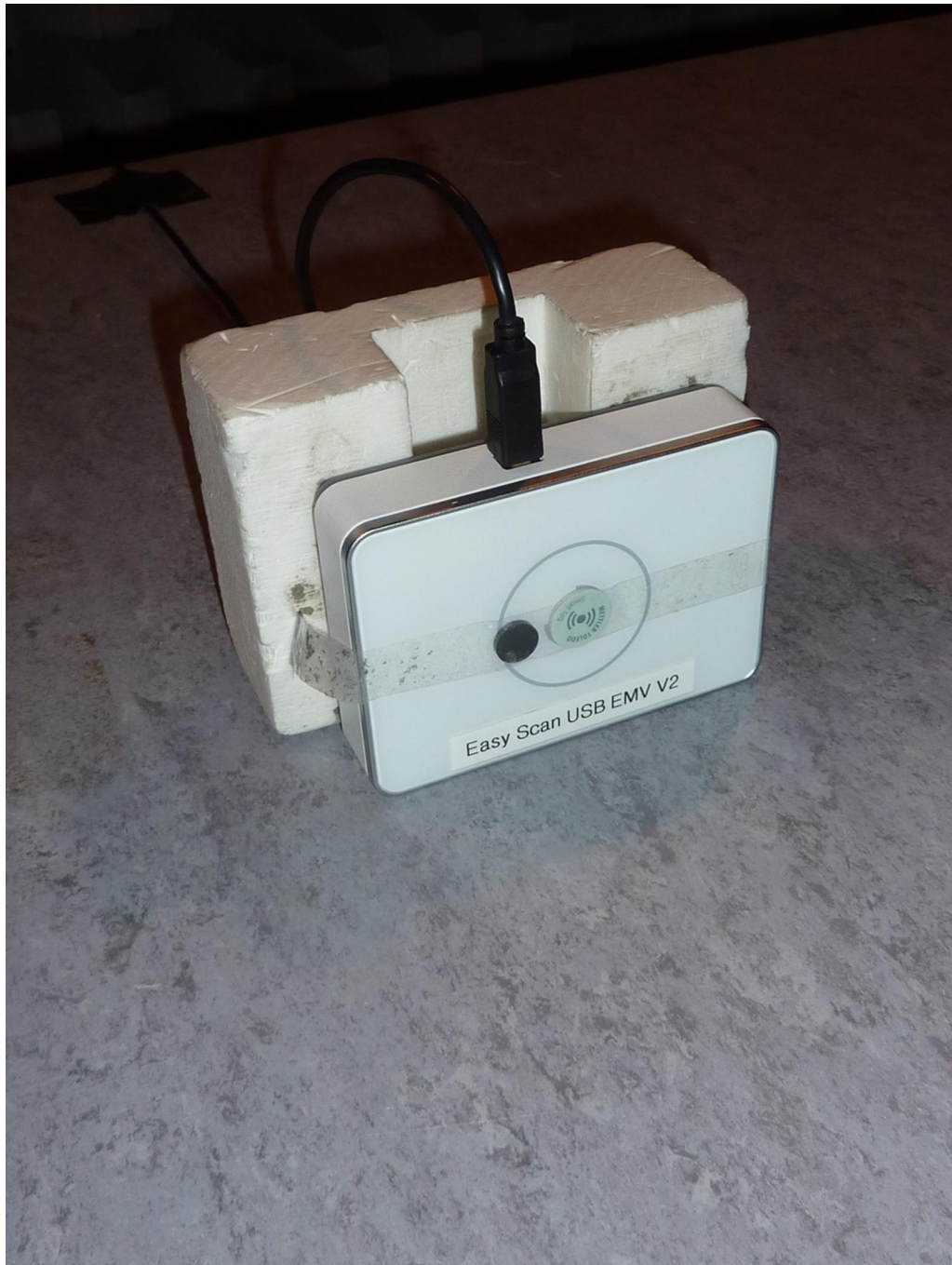
172414_7.jpg: EasyScan USB, test set-up fully anechoic chamber
