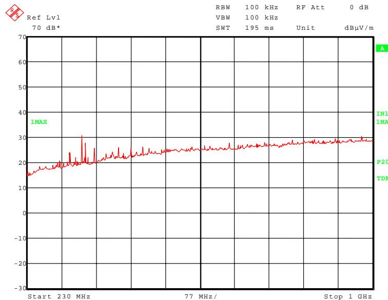
The following frequencies were found emission test outside restricted bands during the preliminary radiated:
