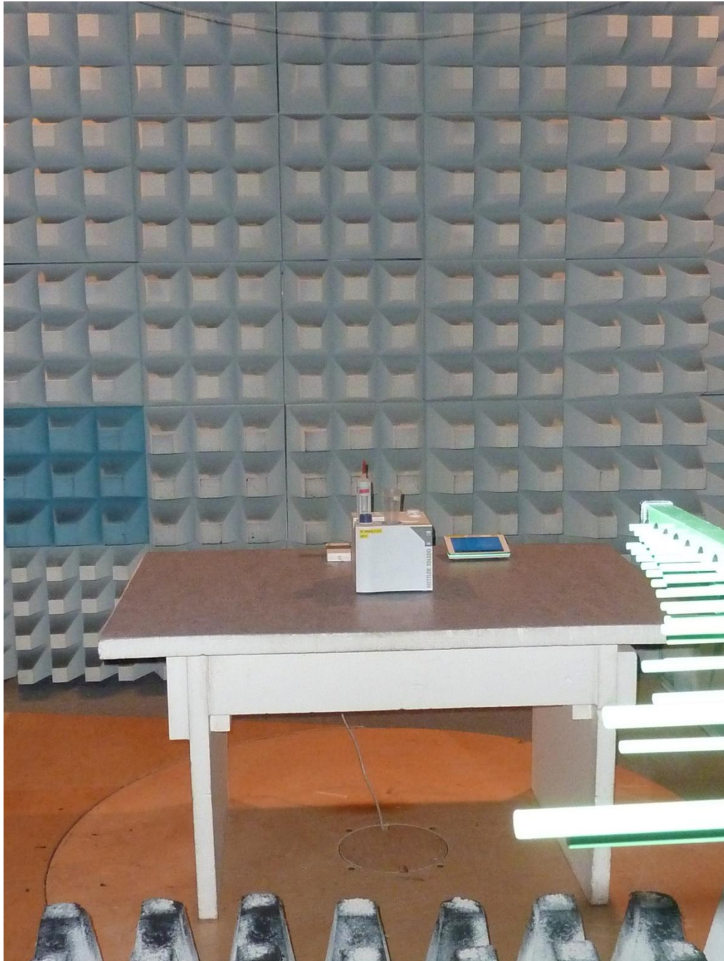
161791emiB3.jpg: Host (Excellence Titrator T9), test setup fully anechoic chamber
