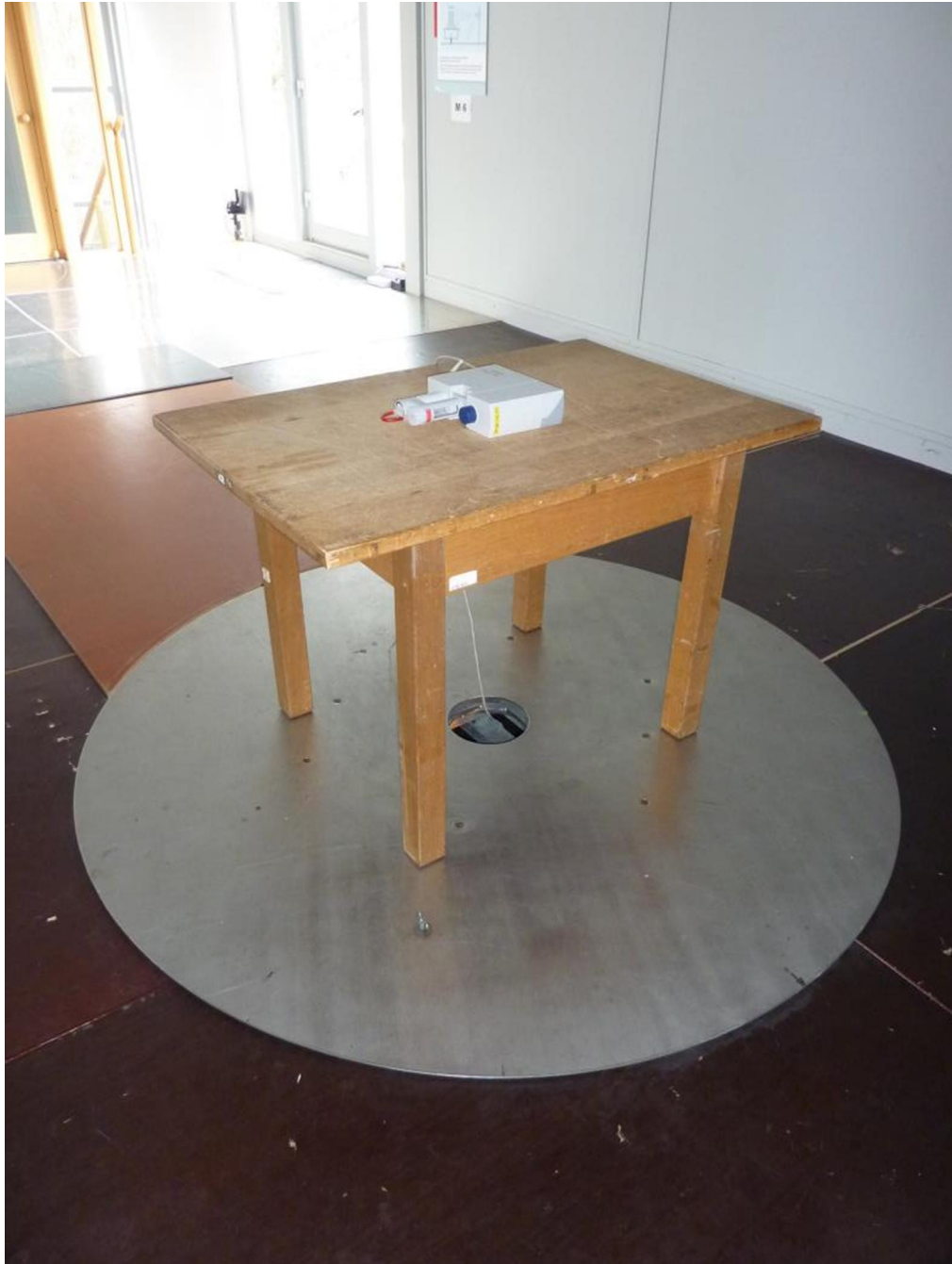
161791emiC5.jpg: Host (Dosing Unit), test setup open area test site position 2
