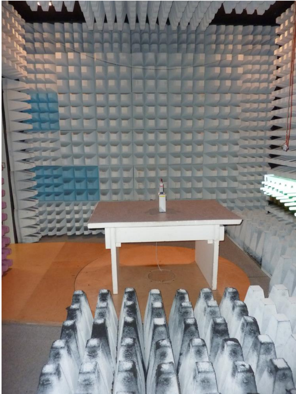
161791emiC2.jpg: Host (Dosing Unit), test setup fully anechoic chamber
