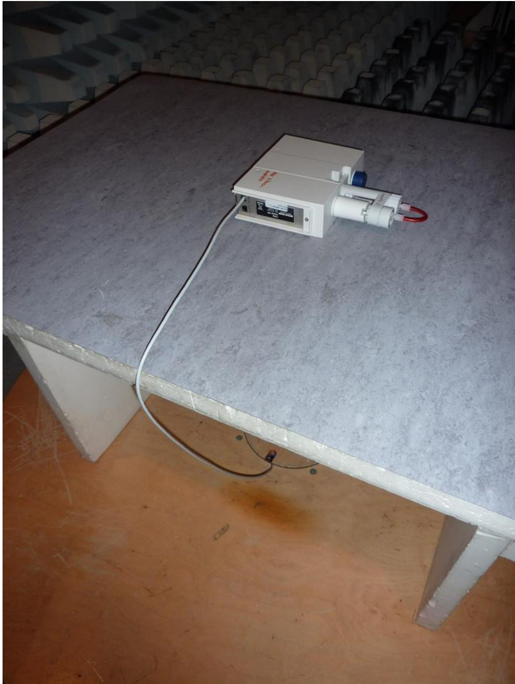
161791emiC3.jpg: Host (Dosing Unit), test setup fully anechoic chamber
