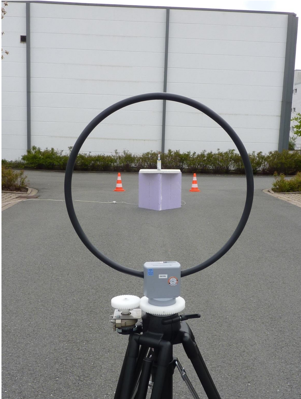
161791emiC6.jpg: Host (Dosing Unit), test setup outdoor test site
