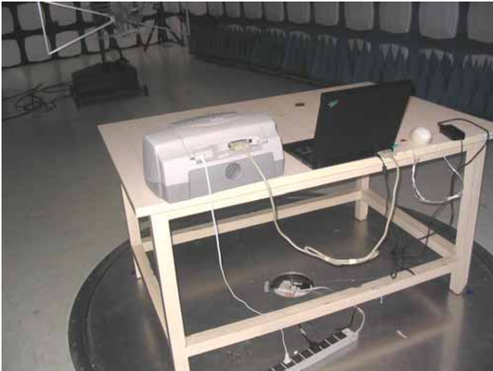
Radiation Emission Test setup
