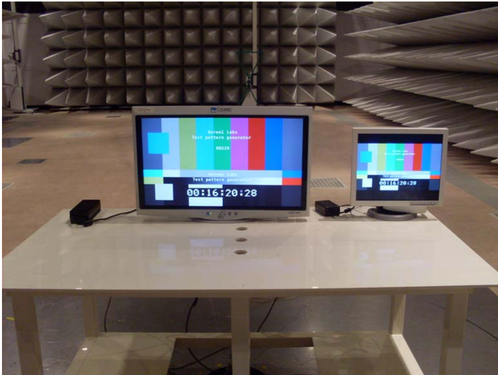
Figure 9, Photo of Radiated emission test setup, 30 MHz to 1000 MHz
