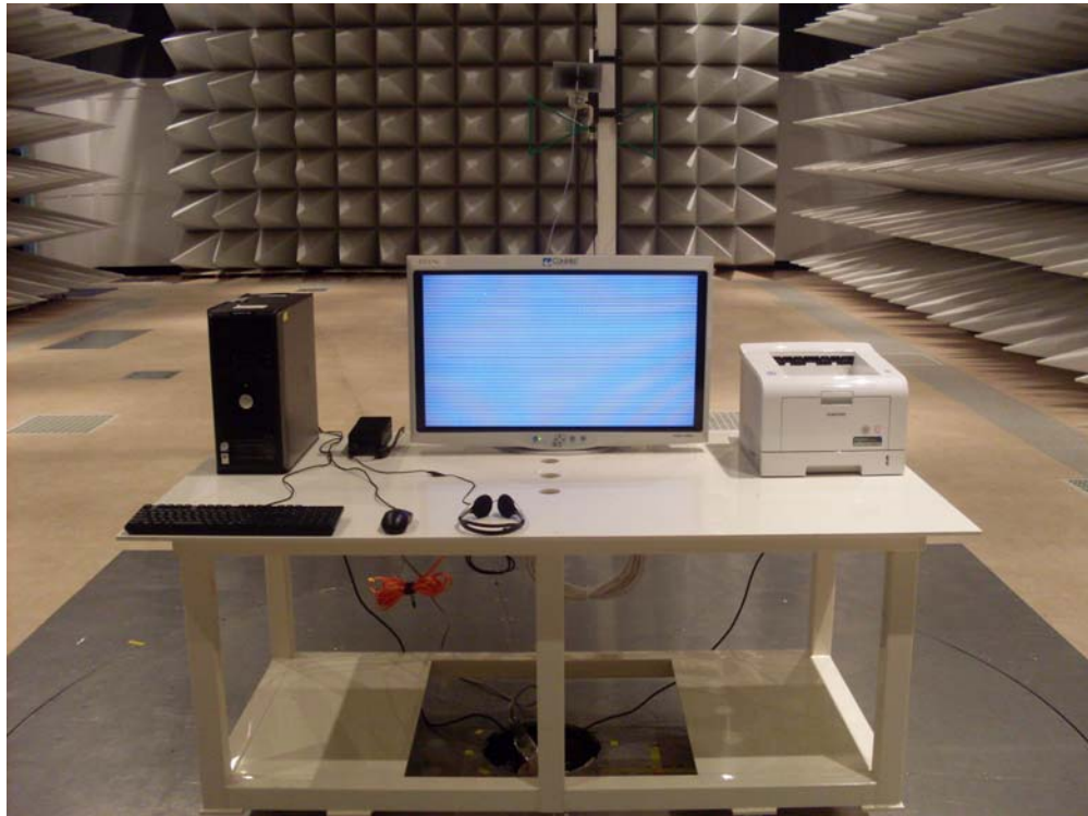
Figure 11, Photo of Radiated emission test setup, 1.0 GHz to 2.0 GHz
