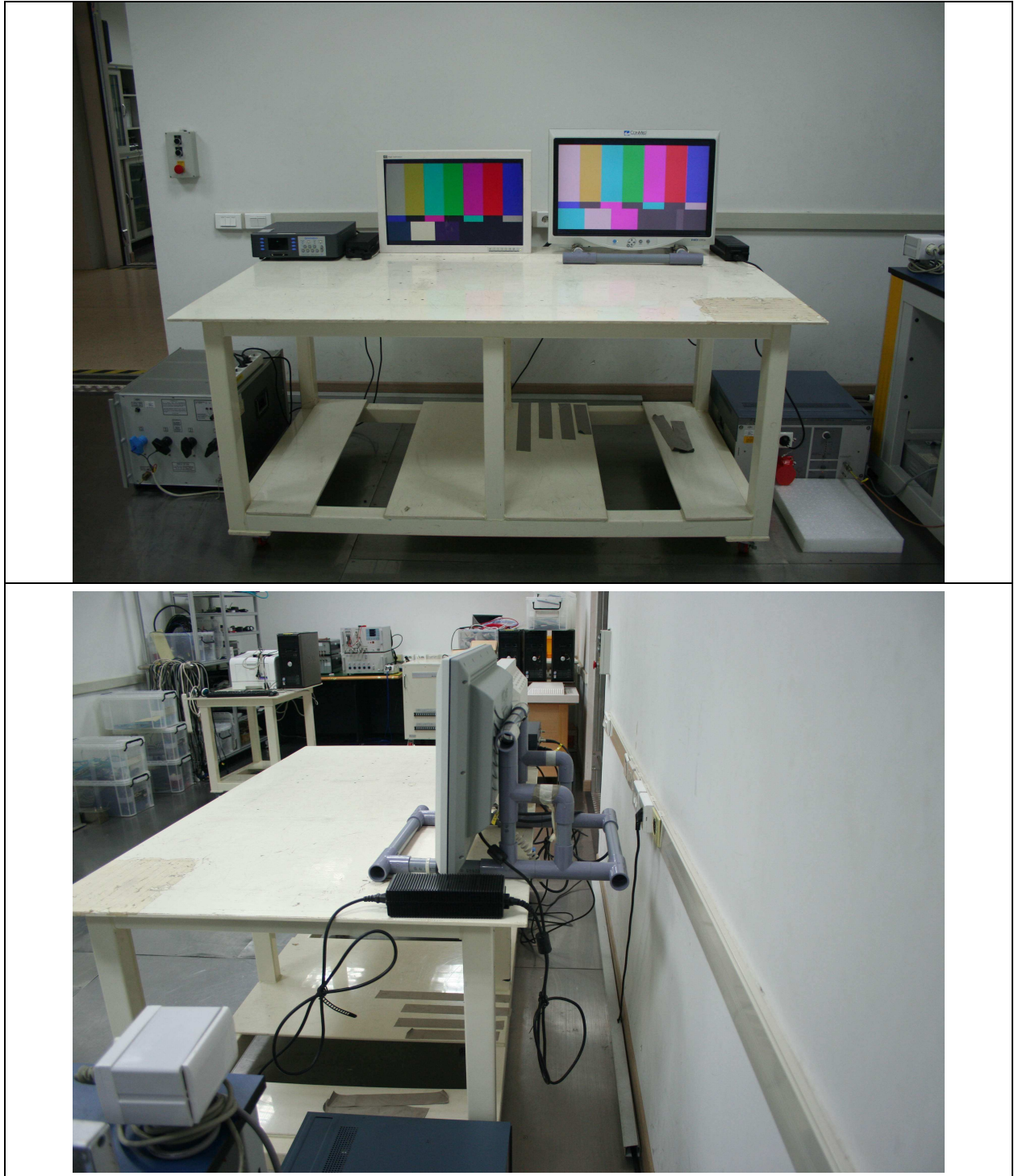
Figure 2. Conducted Emission Test Setup: SDI In/Out Mode
