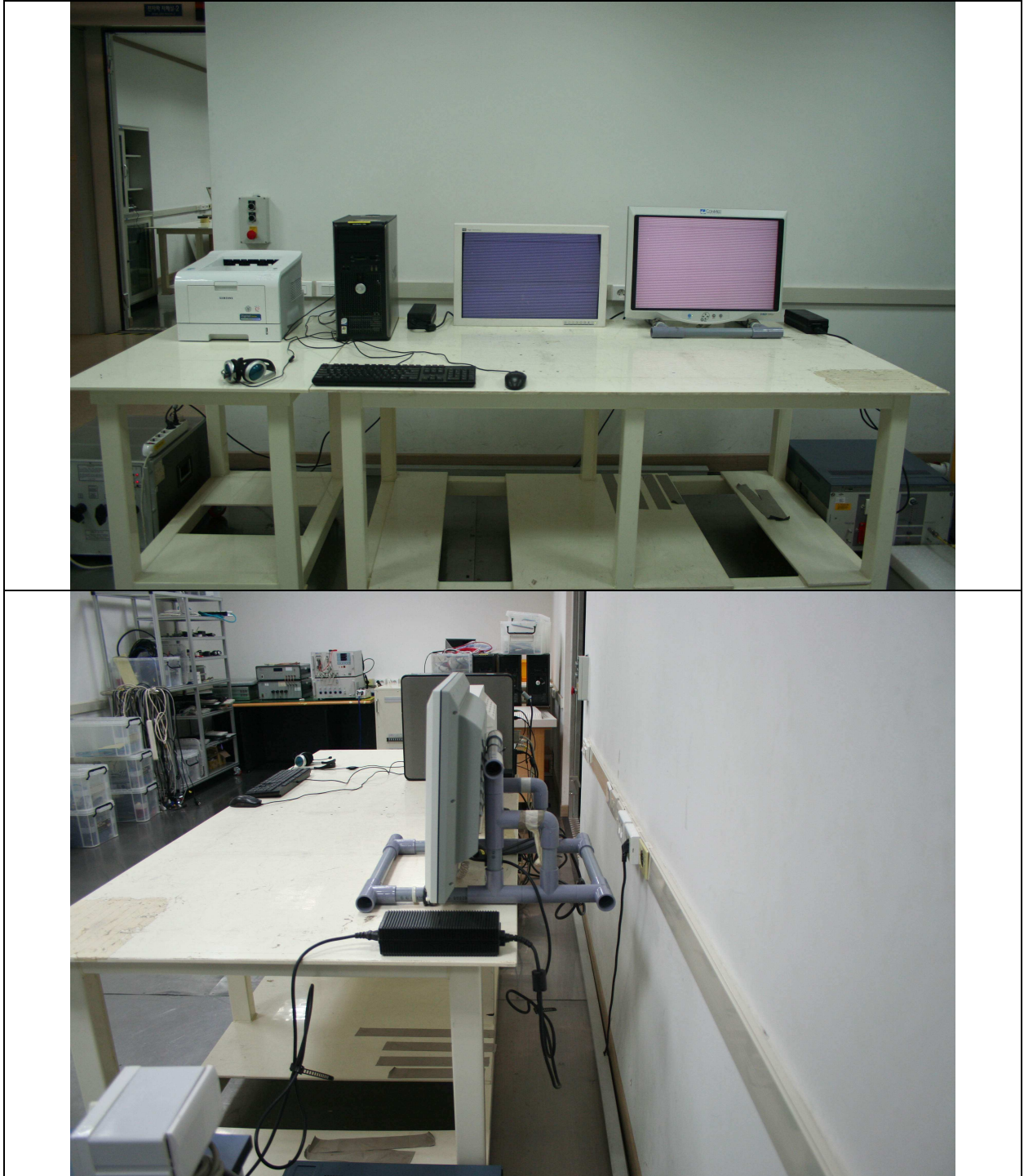
Figure 1. Conducted Emission Test Setup: DVI In/Out Mode
