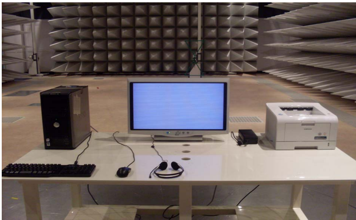
Figure 9, Photo of Radiated emission test setup
