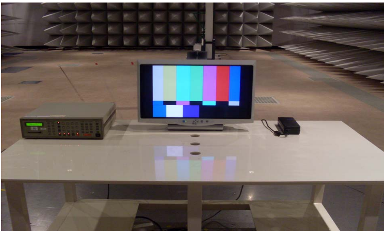
Figure 11, Photo of Radiated emission test setup
