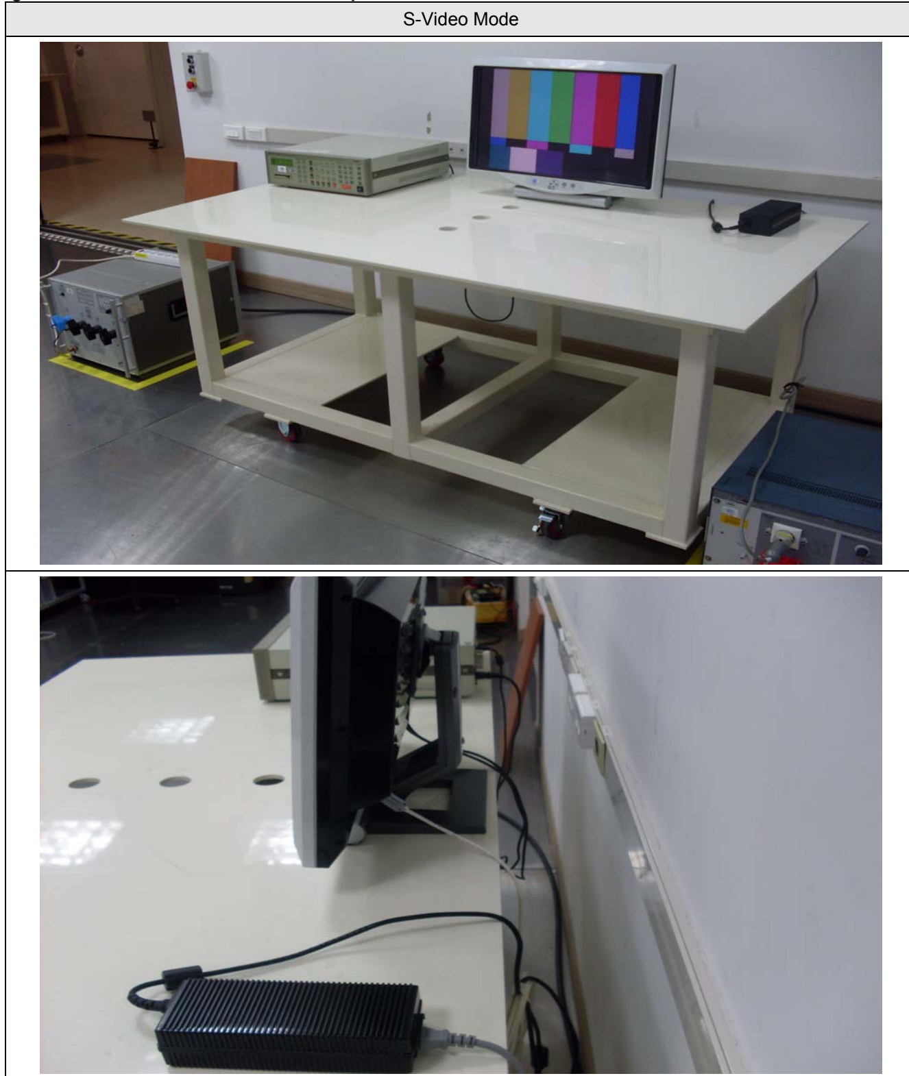
Figure 2. Conducted Emission Test Setup
