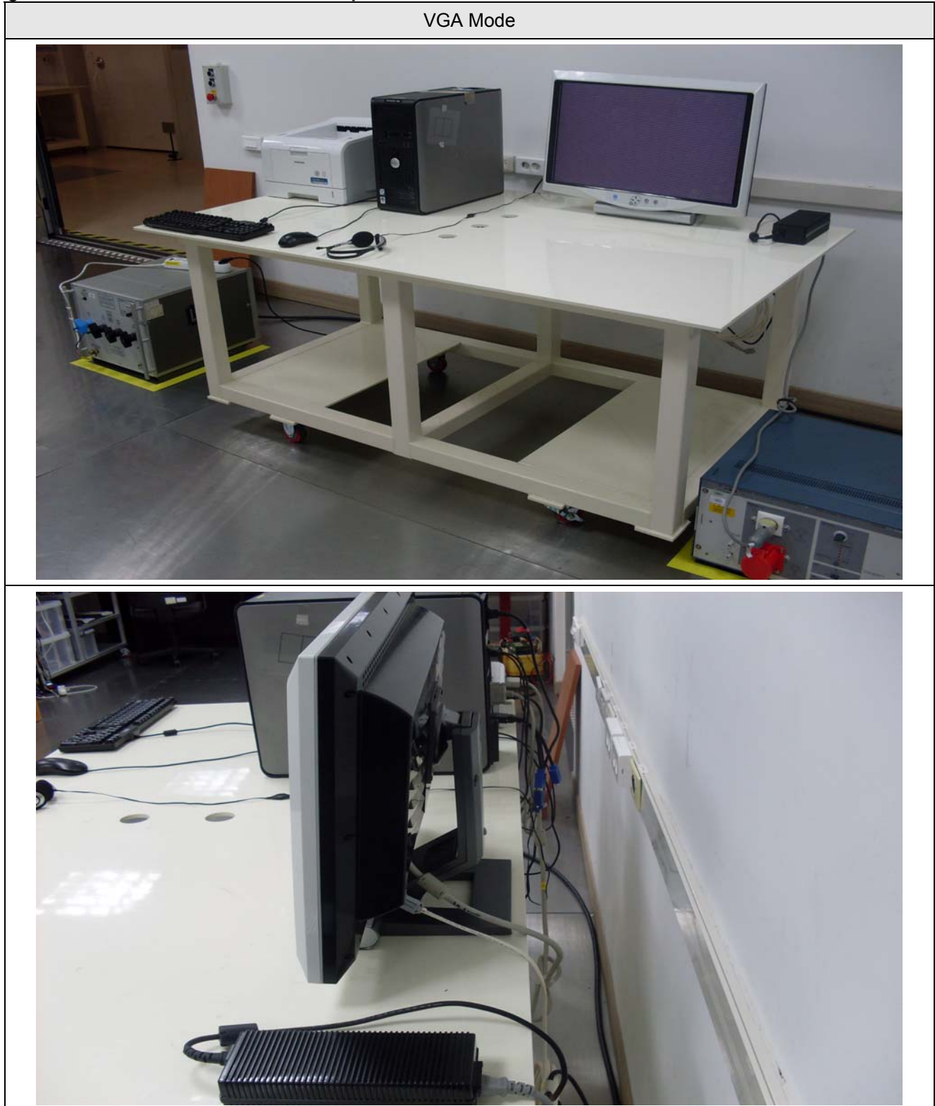
Figure 1. Conducted Emission Test Setup
