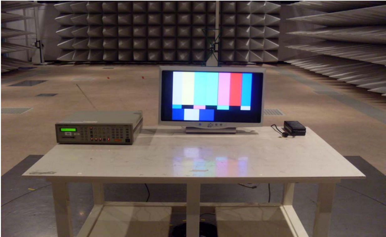
Figure 9, Photo of Radiated emission test setup
