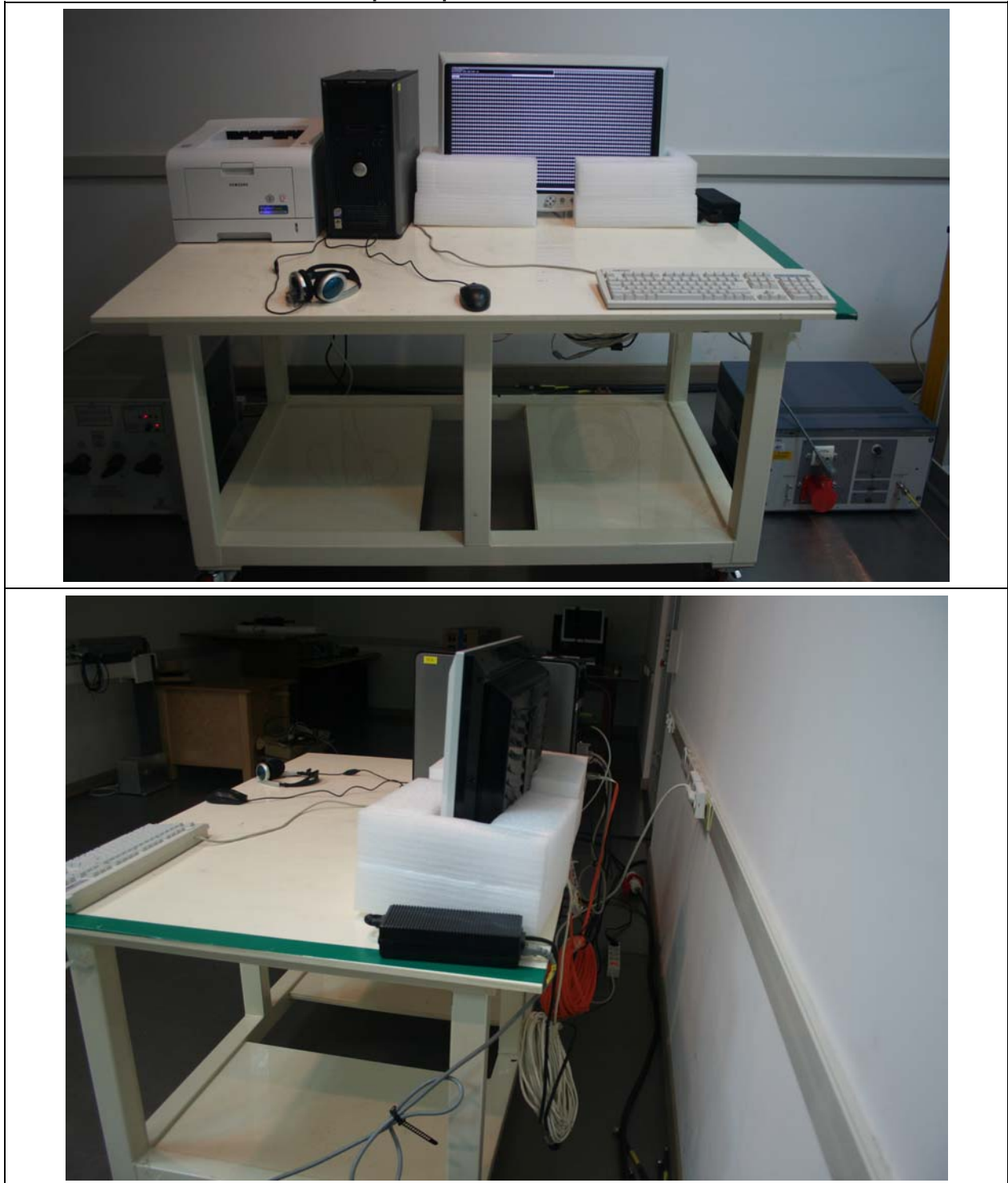
Figure 1. Conducted Emission Test Setup for Optical DVI Mode
