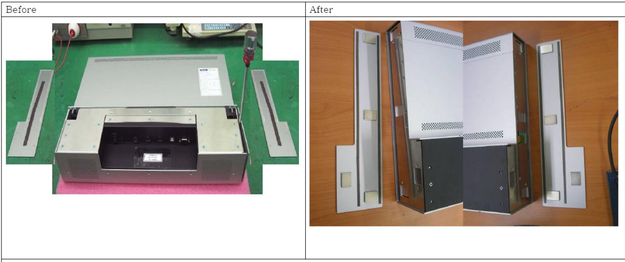
1) Glue point of double stick EMI Tape is changed since the assembly method of the side-plate is changed.
