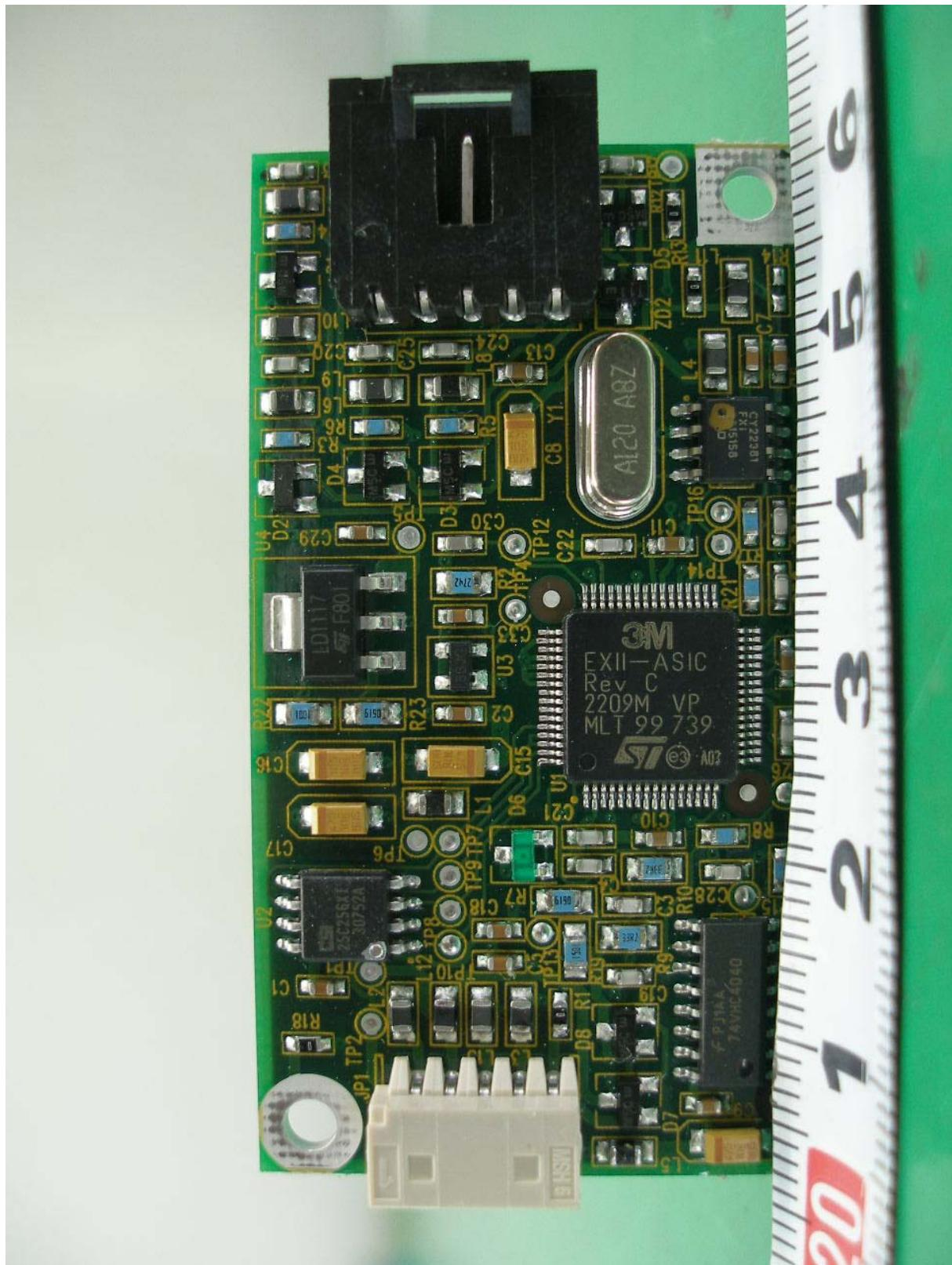
● Rear View of USB Controller Board
