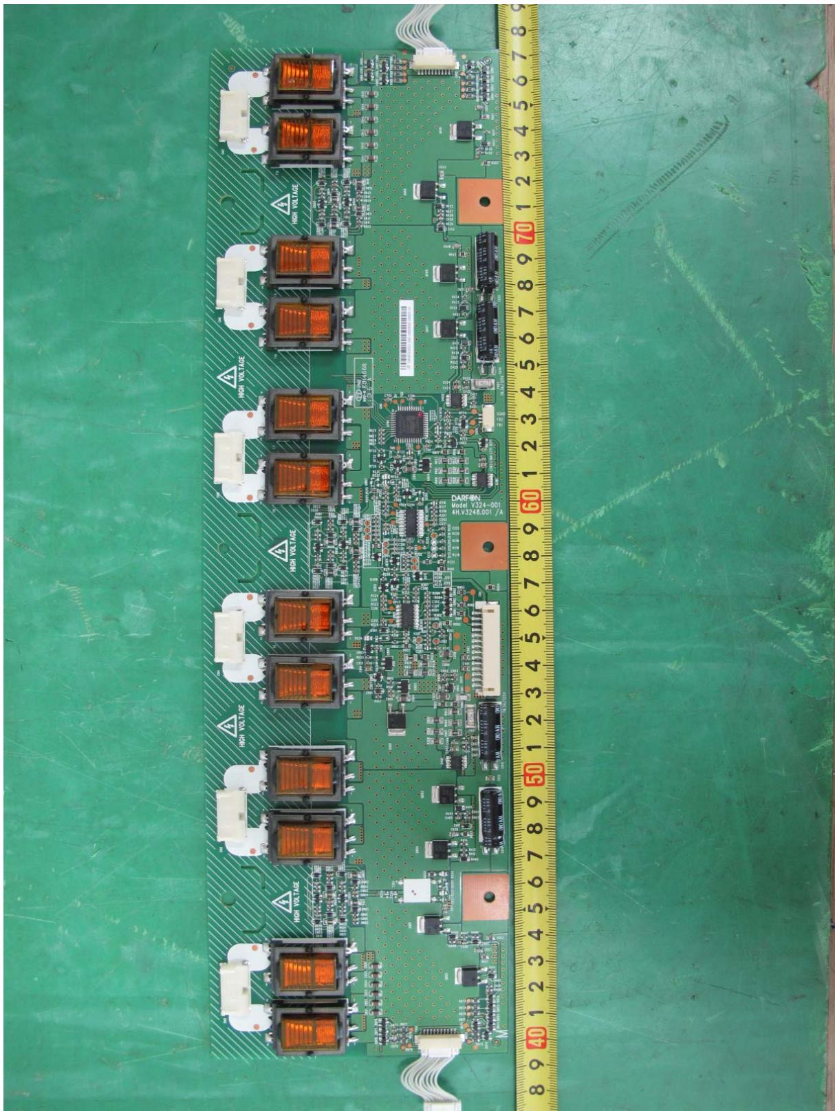
● Rear View of Inverter Board V324-001(M)
