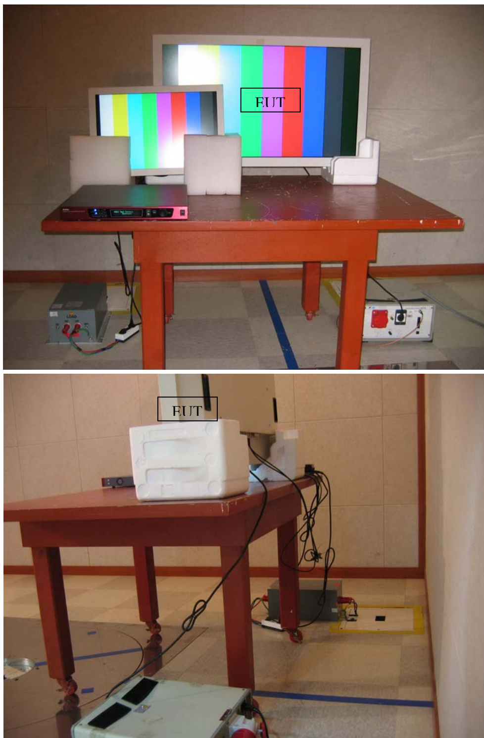
Figure 2 Conducted Emission Test Setup: SDI Mode
