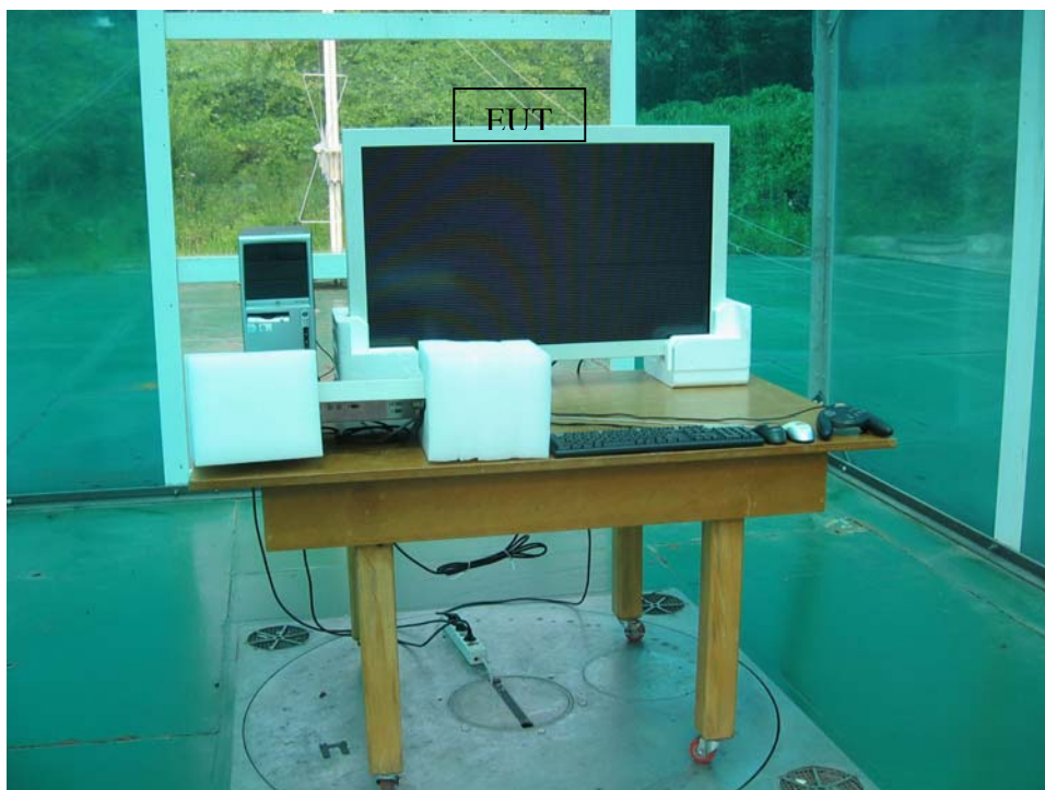
Figure 5 Photo of Radiated emission test setup: DVI Mode
