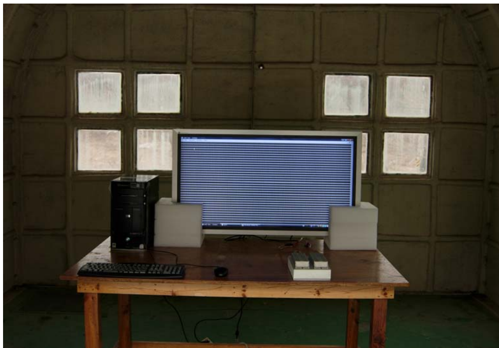
Photo of Radiated emission test setup: DVI/DSUB Mode
