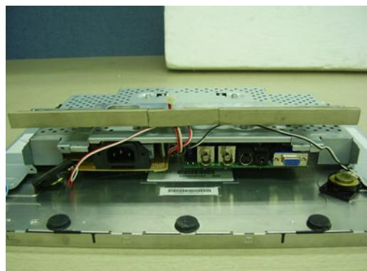
Conductive tape and Gaskets are applied to the panel and the bottom of the chassis.
