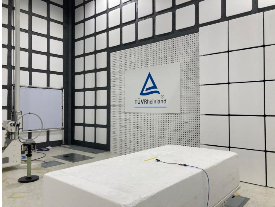
Photograph 3: Test Setup for Spurious Emissions (Back View 1)
