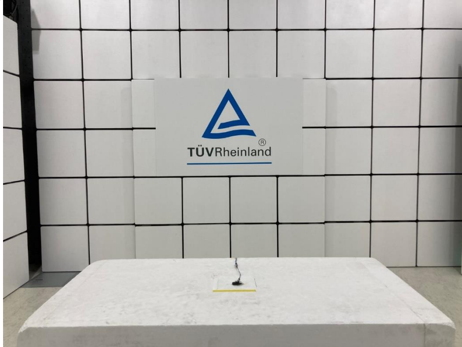
Photograph 1: Test Setup for Spurious Emissions (Front View 1)
