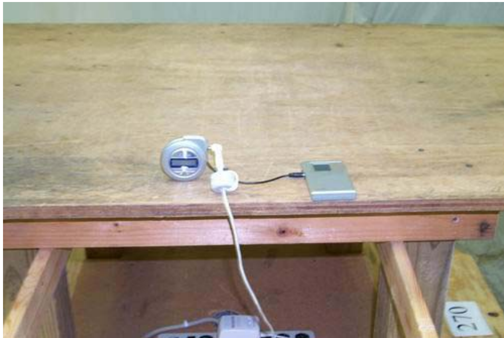
Figure 3.4 Radiated Test Setup, position 1-X (DC Power)
