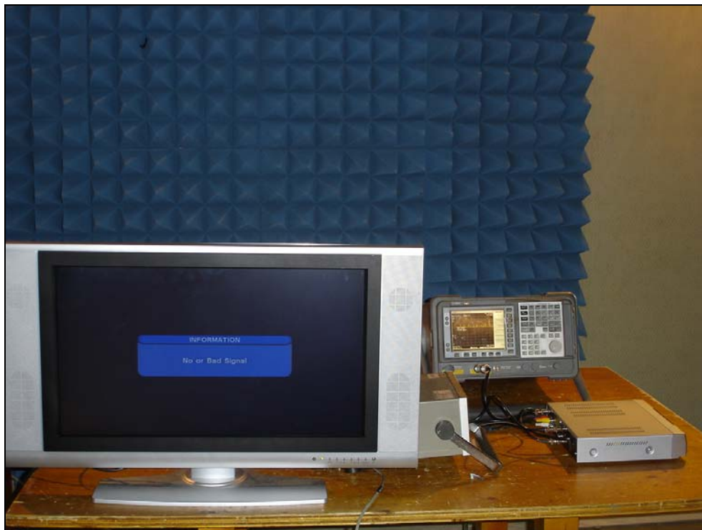
Photograph 3: Setup for Antenna-Conducted Power Measurements
