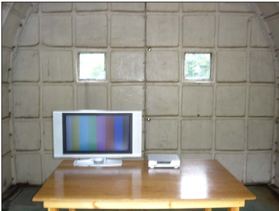
Photograph 2: Setup for Radiated Emissions
