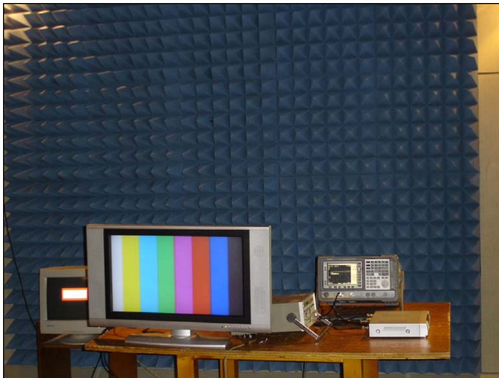
Photograph 4: Setup for Output Signal Conducted Level Measurement
