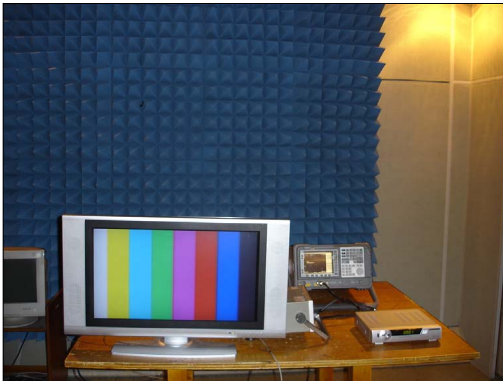
Photograph 6: Setup for Antenna Transfer Switch Measurement
