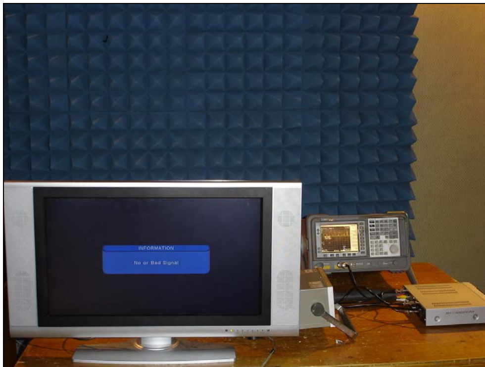
Photograph 3: Setup for Antenna-Conducted Power Measurements
