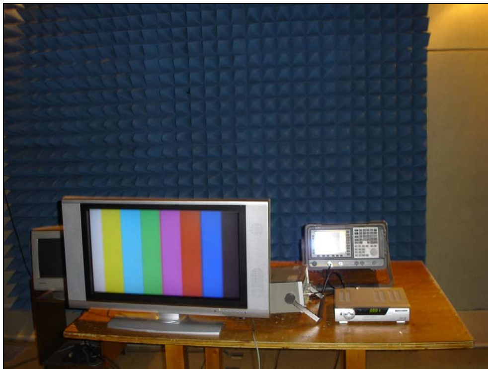
Photograph 5: Setup for Output Terminal conducted Spurious Emission Measurement
