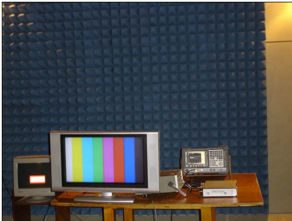
Photograph 4: Setup for Output Signal Conducted Level Measurement
