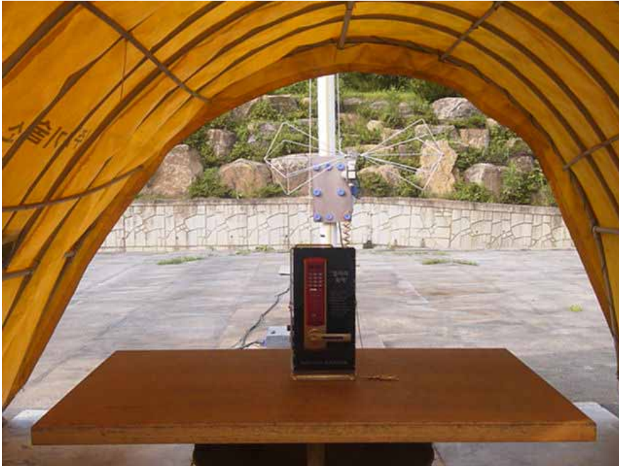
Photograph 1 : Setup for radiated Emissions
