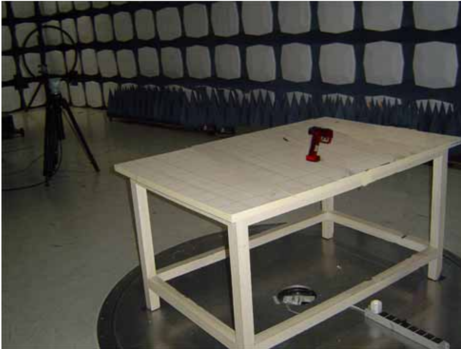
Radiation Emission Test setup
