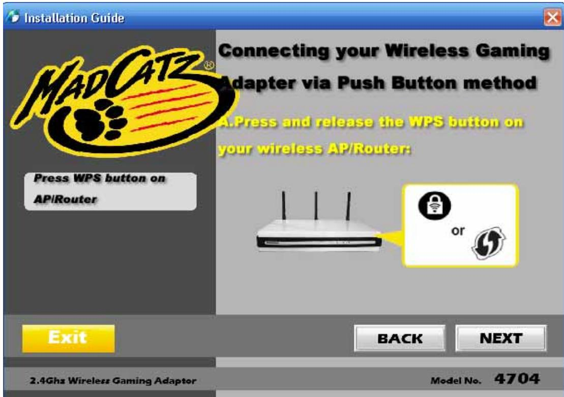
B. Within 2 minutes of pressing the WPS button on your wireless AP/Router, press and release the Wireless Gaming Adapter's WPS button as pictured below:
