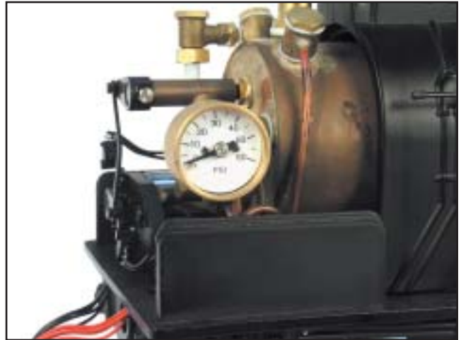
fig. #20a Locomotive pressure gauge
