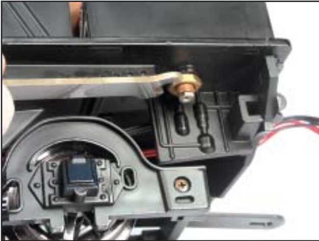
fig. #20 Drain cock valve
