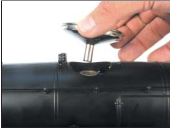
fig. #11 Metal funnel placed in locomotive
