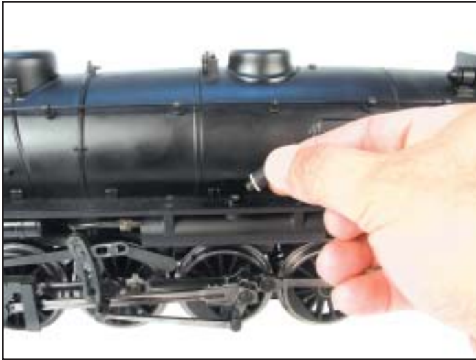
fig. #8 Removing the oil valve
