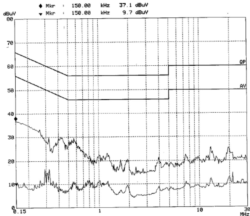
Conduction Disturbance Test
