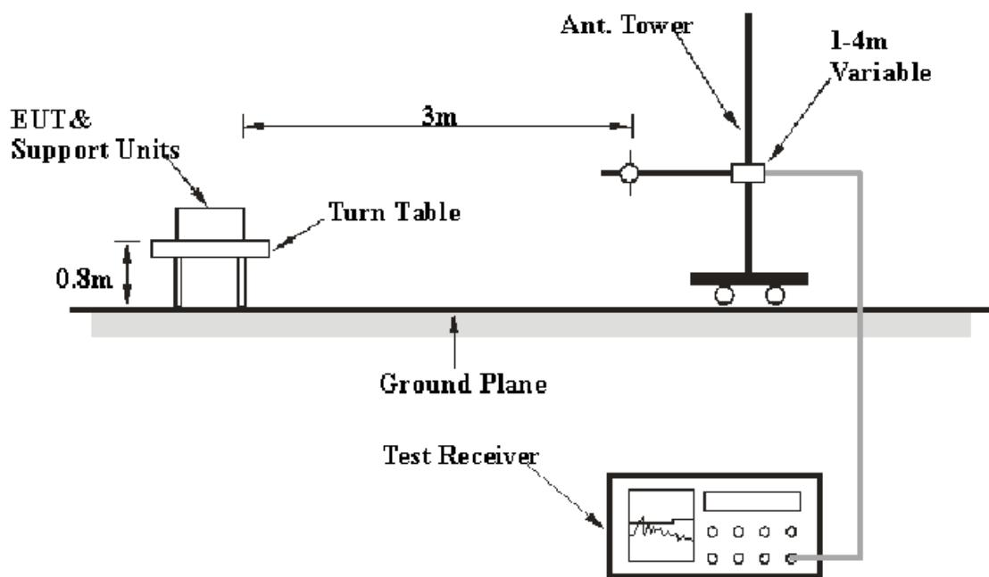
The radiated emission tests were performed in the chamber B test site, using the setup accordance with the ANSI C63.4-2003. The specification used was the FCC 15.209 and 15.235 limits.
