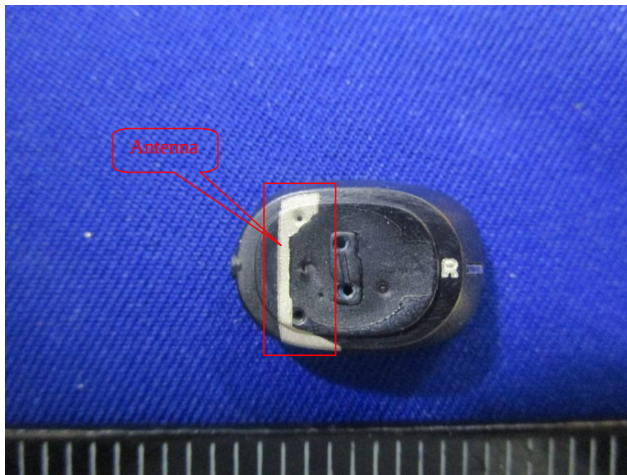
EUT – Right Earbud Antenna View
