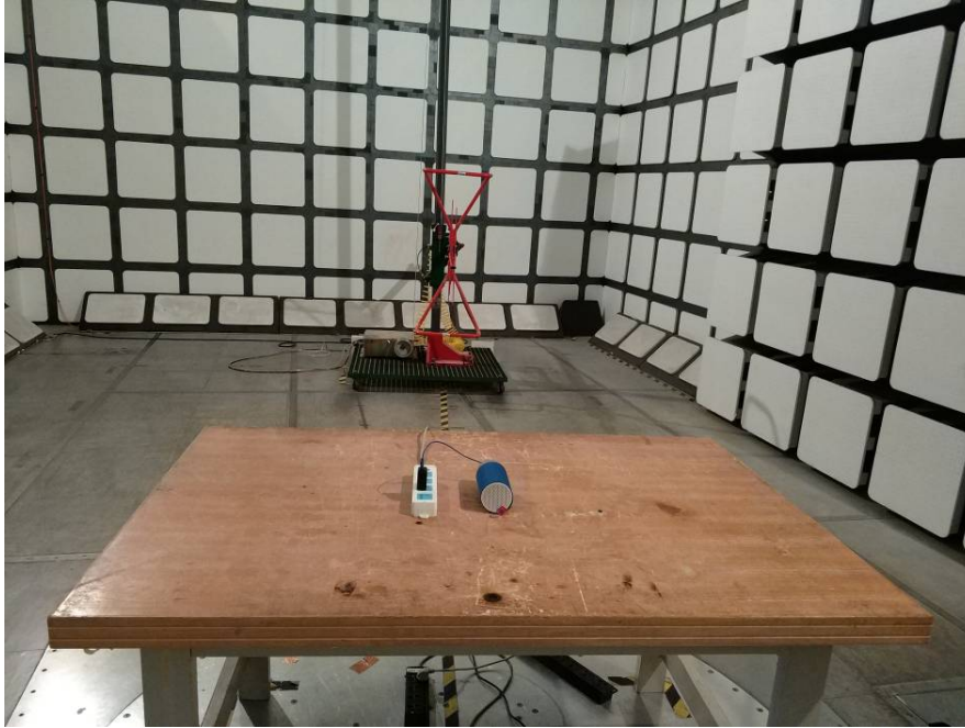
Radiated Emissions View (Below 1 GHz)
