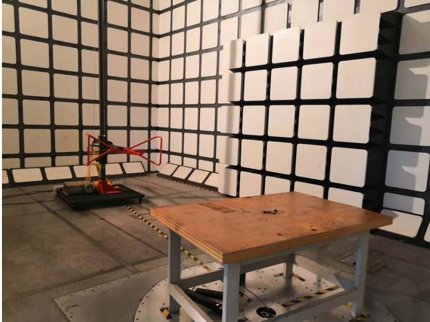
Radiated Emissions View (Below 1 GHz)
