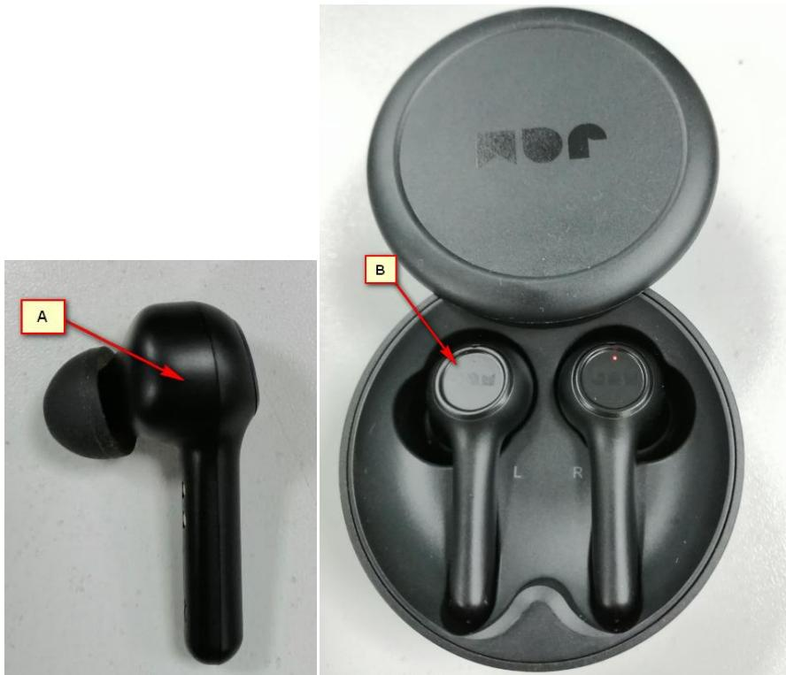
Conclusion: Based on the above description of area A to B, we conclude that the device is unquestionably too small for enabling the FCC ID to be printed onto any surface. We therefore request to move the FCC ID to the user manual and charging case.
