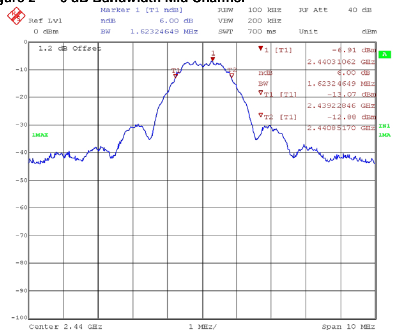
Figure 2 6 dB Bandwidth Mid Channel
