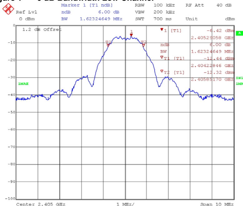
Figure 1 6 dB Bandwidth Low Channel
