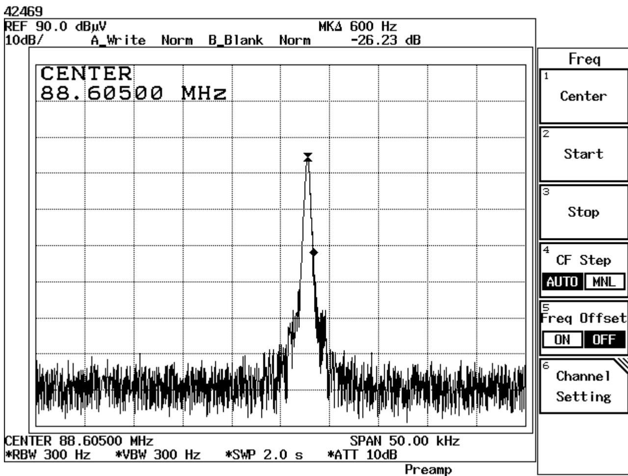
Result : The field strength of any emission within the operation band did not exceed 48 dB( $\mu$ V/m) for average value or 68 dB( $\mu$ V/m) for peak value. Refer to page 9 for the recorded value for the emission at the fundamental frequency.
