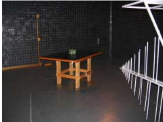
Photograph 9.2.1 Setup for radiated emission measurements, below 1 GHz
