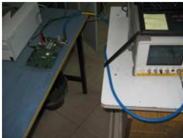
Photograph 7.2.2 Occupied bandwidth test setup
