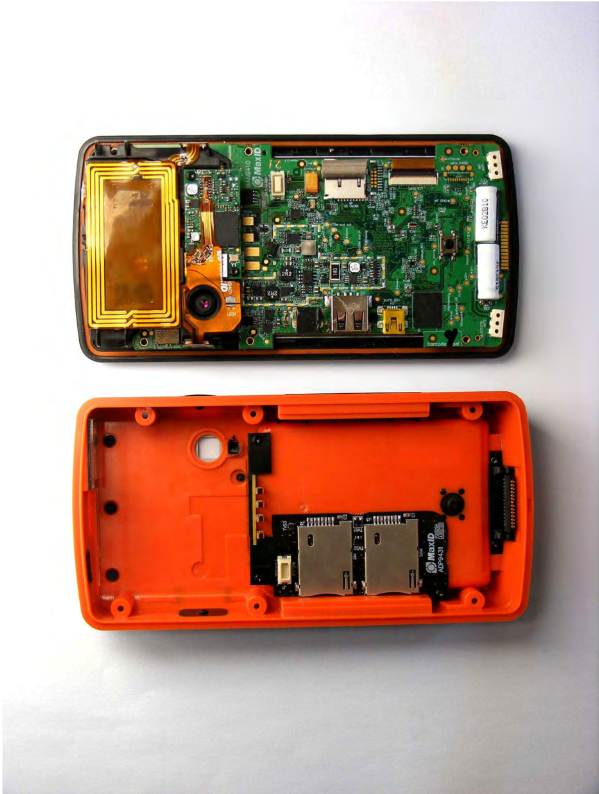
Figure 9: iDL300 top and bottom assembly opened
