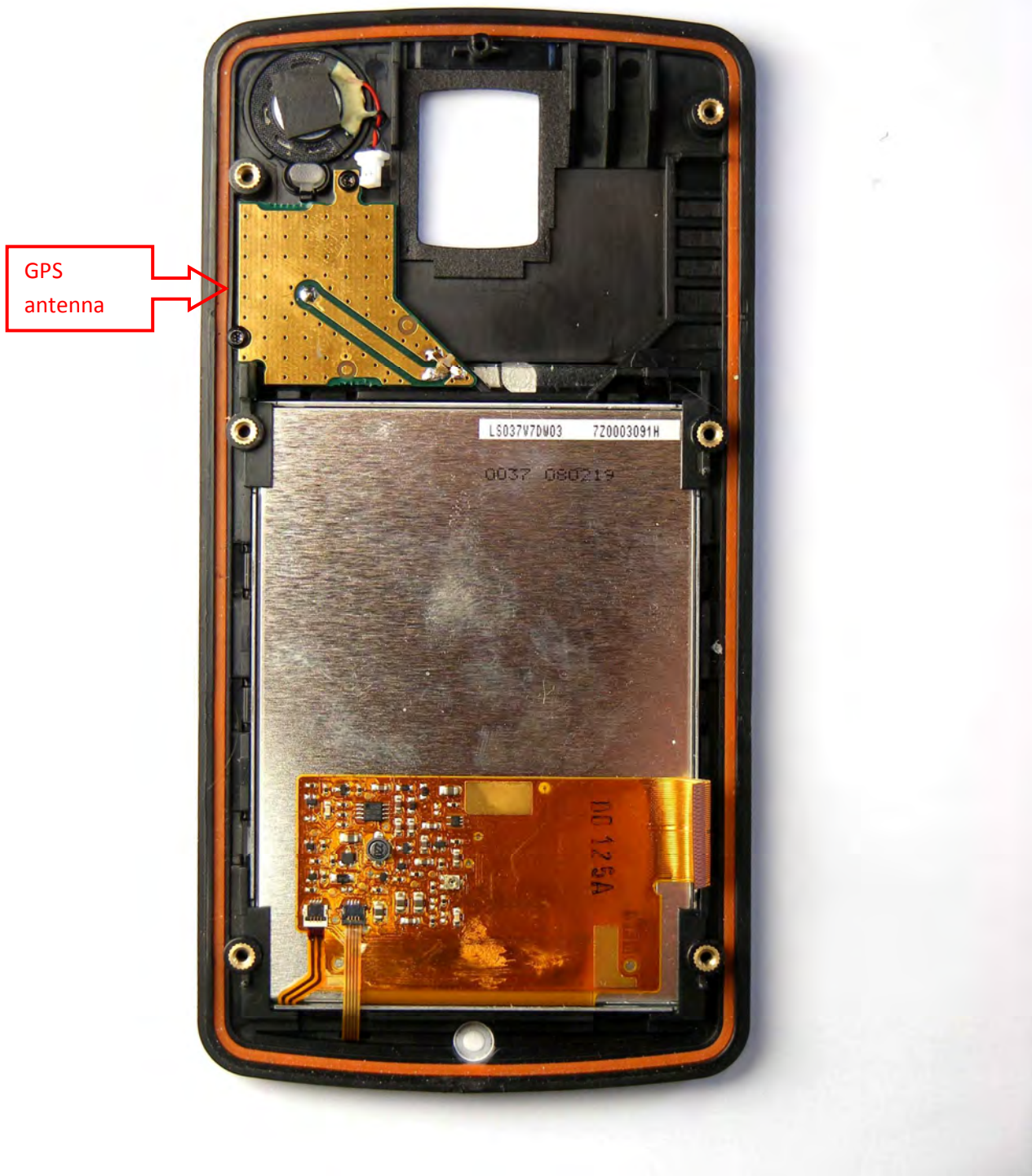
Figure4: iDL300 top assembly with LCD, GPS antenna and speaker
