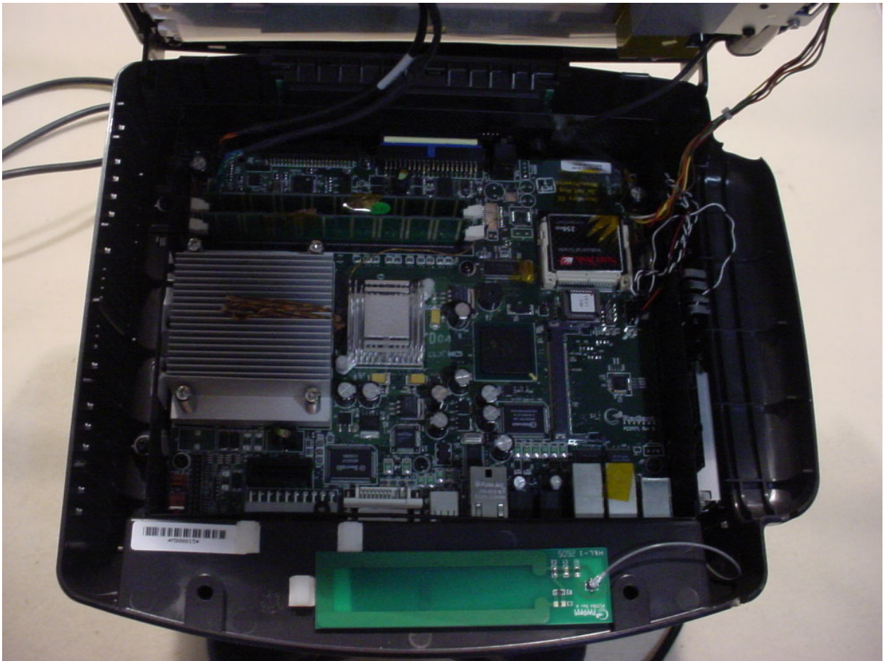
Figure 2: Inside View Showing Motherboard and Antenna
